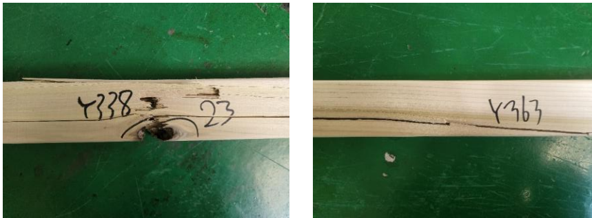
Fig. 4. Cause of tensile failure (left: knot, right: grain angle)
