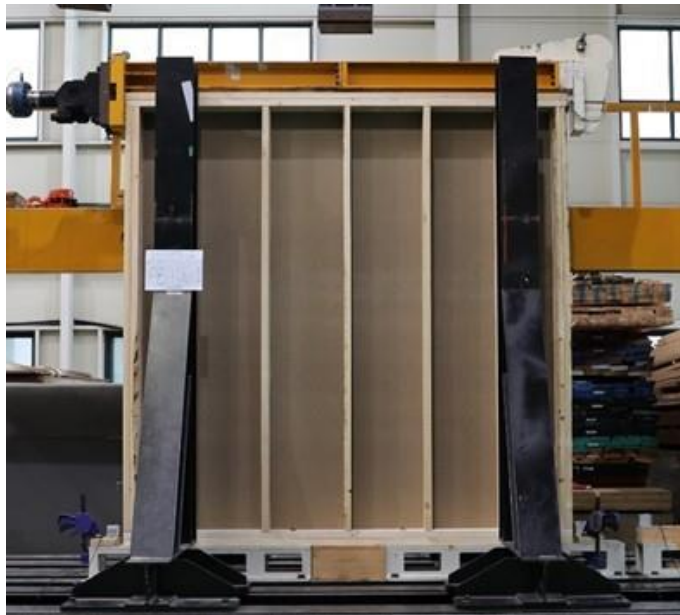
(b) Test picture of Structural PB light-frame wall
