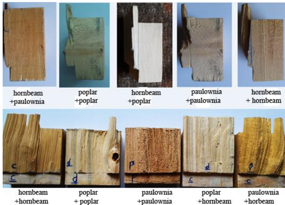
Fig. 4. Failure modes of specimens in shear block test in dry condition
