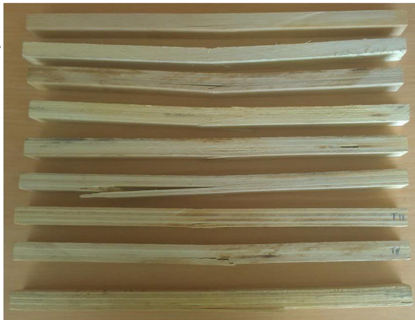
Fig. 3. The failure mode pictures from the MOR tests and the analysis of the differences in failure modes between different LVL specimens
