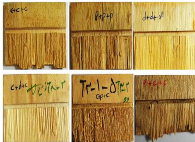
Fig. 5. Failure modes of LVL specimens in shear strength test
