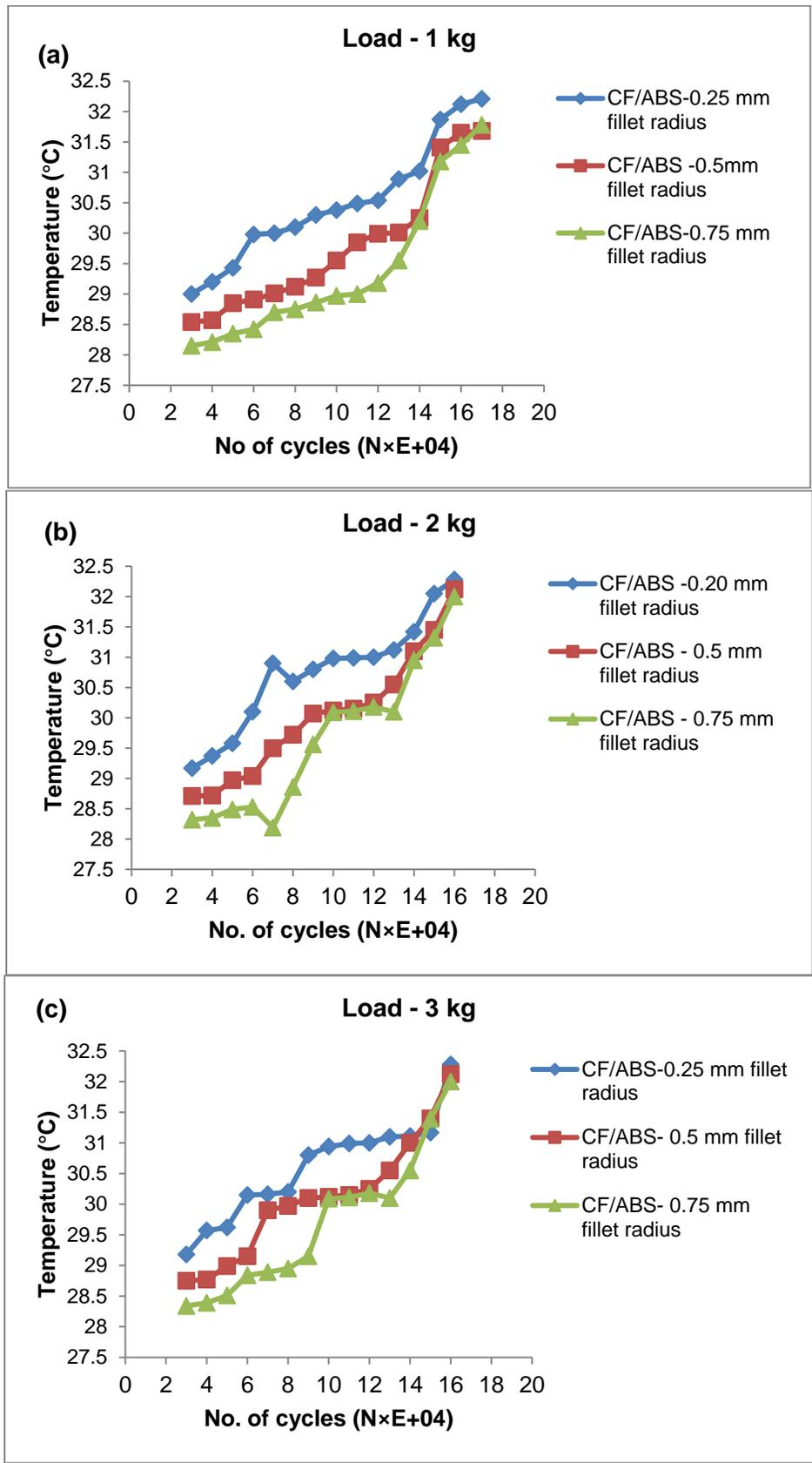
**Fig. 5.** Temperatures of CF/ABS gears with different fillet radii at life cycle runs under (a) 1, (b) 2 and (c) 3 kg loads
