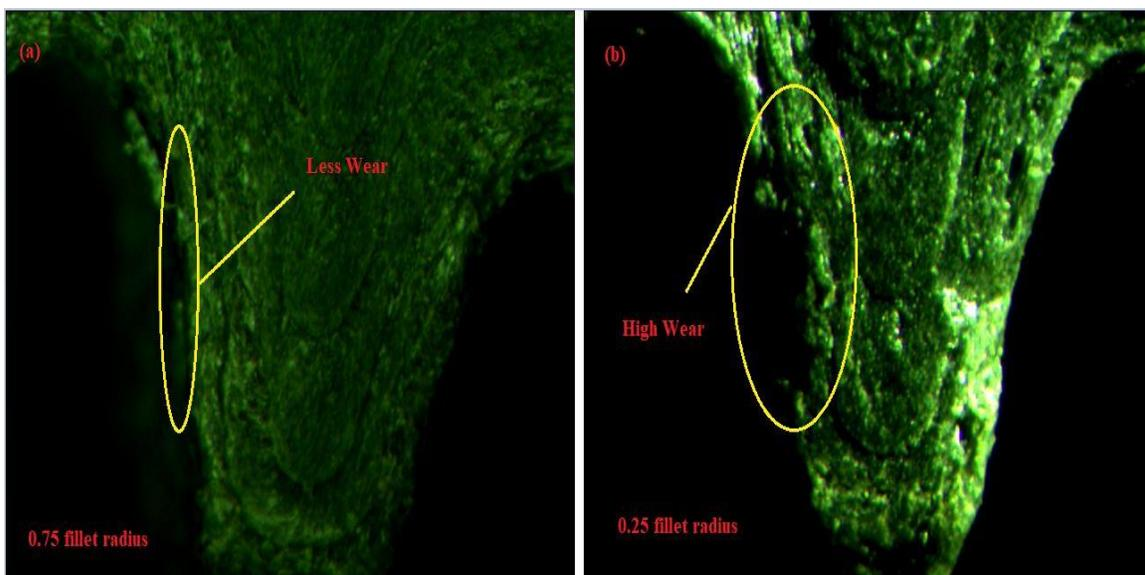
**Fig. 3.** Micrographic analysis of gear fillet radii of (a) 0.75 and (b) 0.25 mm
