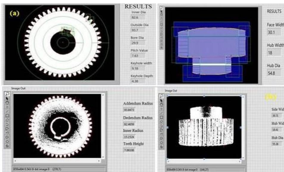
Fig. 1. 3D-printed (a) ABS and (b) CF/ABS spur gears and their machine visions
