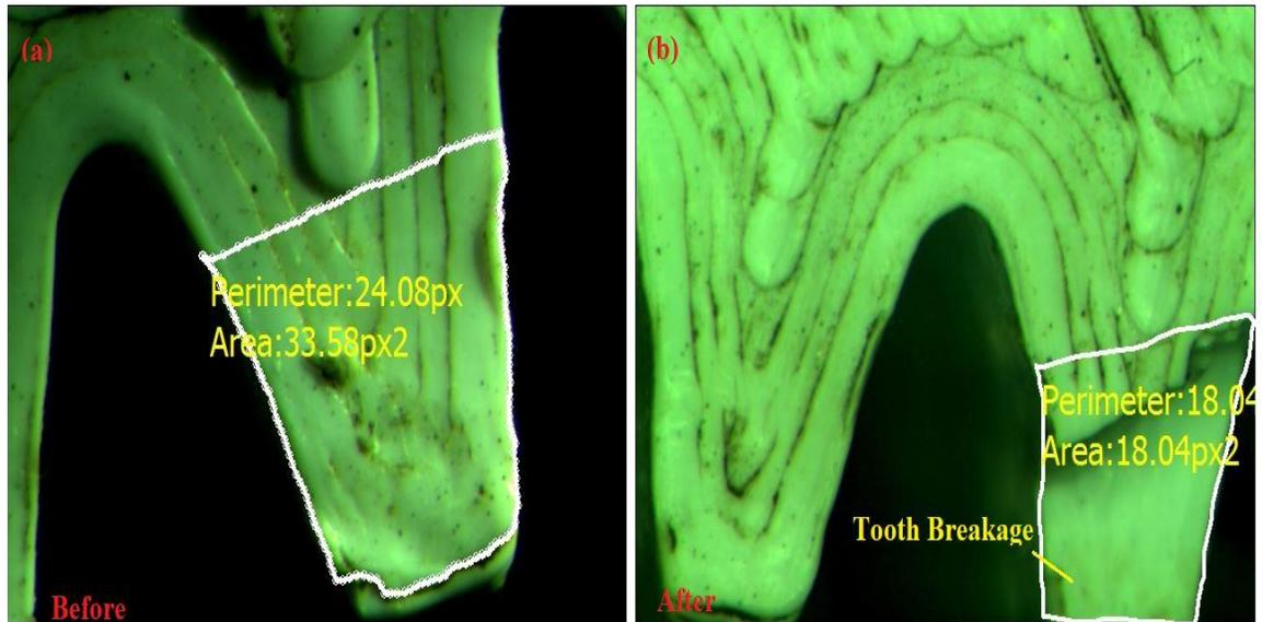
Fig. 6. ABS with fillet radius of 0.50 mm (a) before and (b) after running
