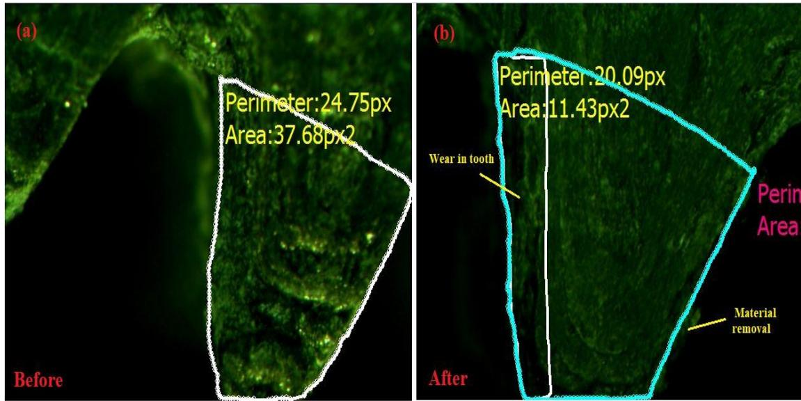
**Fig. 8.** CF/ABS with fillet radius of 0.25 mm(a) before and (b) after running
