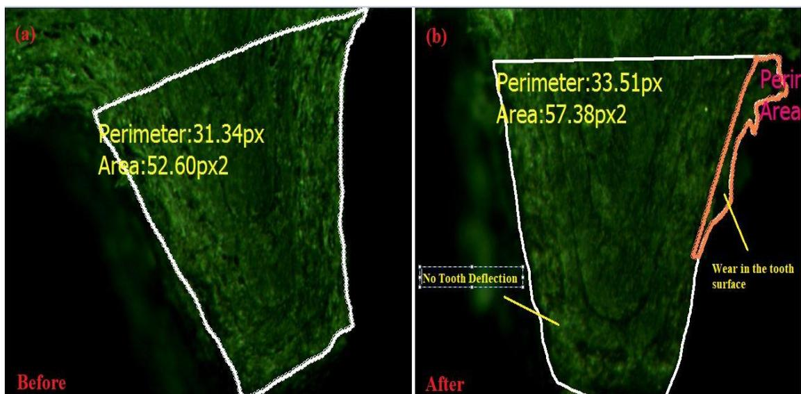
Fig. 7. CF/ABS with fillet radius of 0.50 mm (a) before and (b) after running
