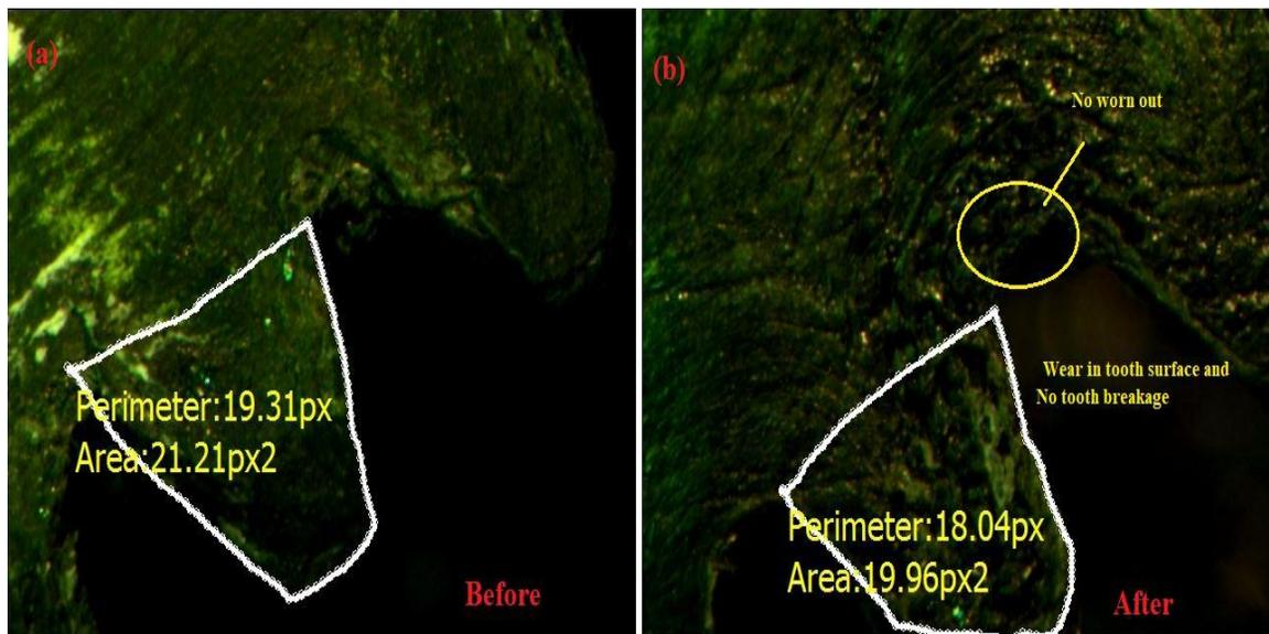
**Fig. 9.** CF/ABS with fillet radius of 0.75 mm(a) before and (b) after running
