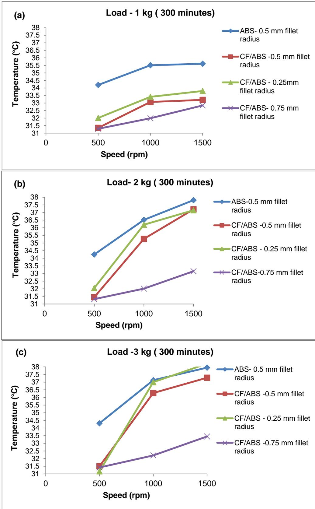
**Fig. 4.** Variation of loads and speeds *versus* temperatures of ABS and CF/ABS gear under (a) 1, (b) 2. and (c) 3 kg loads for 300 min
