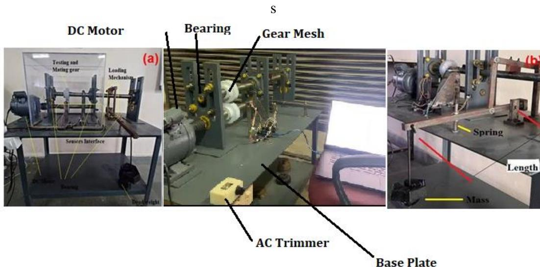
**Fig. 2.** (a) Gear test rig set-up and (b) its loading mechanism
