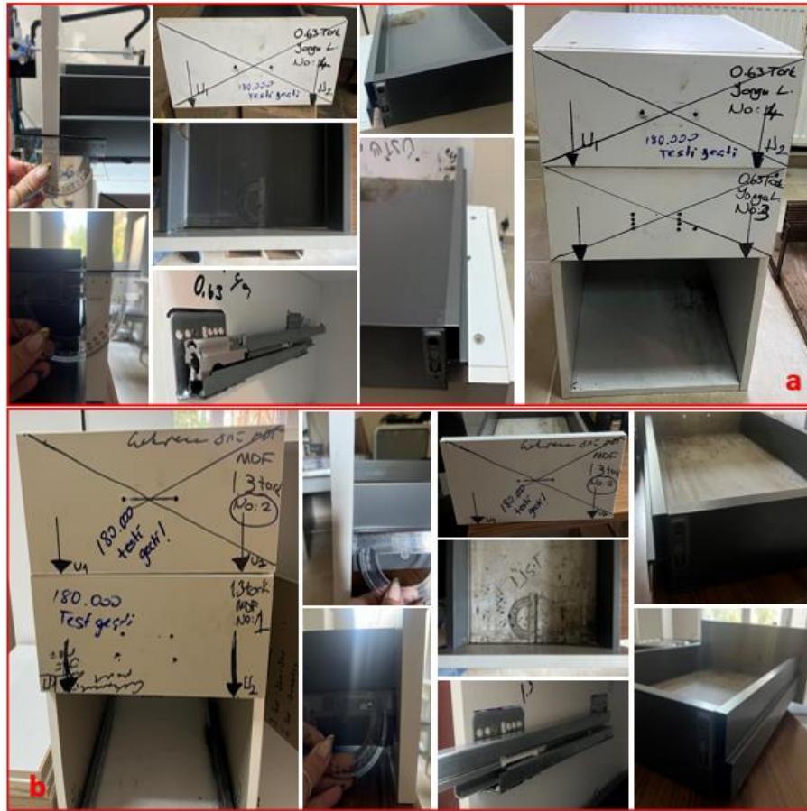
Fig. 6. Typical deformation (a) PB drawers from 0.63N/m torque, (b) MDF drawers from 1.3N/m torque
