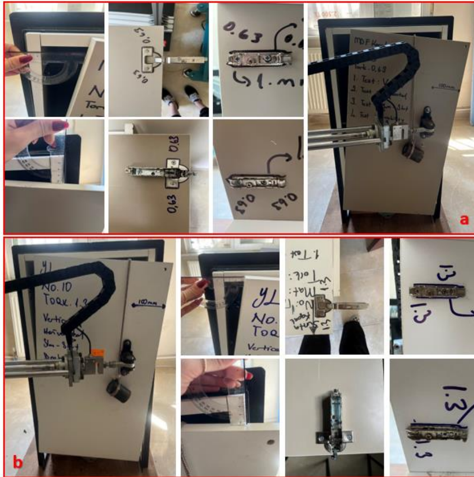
Fig. 5. Typical deformation (a) MDF doors from 0.63N/m torque, (b) PB doors from 1.3N/m torque
