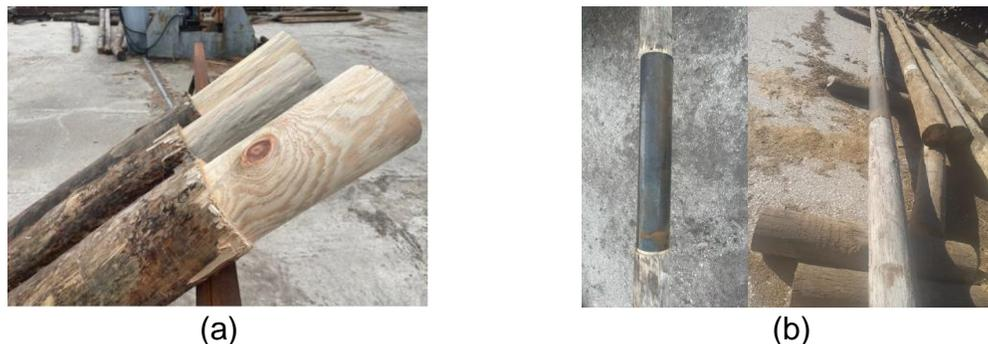
**Fig. 5.** The wooden poles (a) before insertion; and (b) with the cylindrical steel tube
