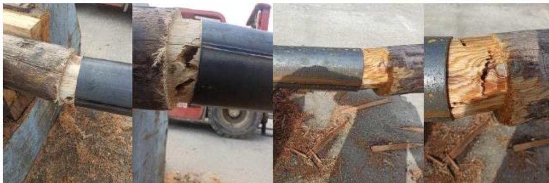
**Fig. 9.** Ruptures observed in the wooden elements inserted in the steel tube
