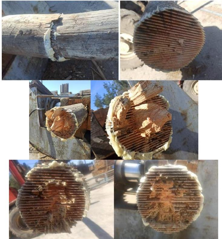
**Fig. 10.** Ruptures observed in the finger joint connections
