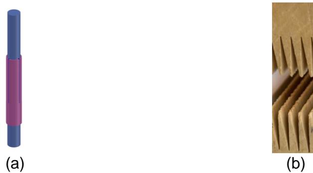
**Fig. 4.** Studied solutions: (a) wood pole members inserted in a cylindrical steel tube; and (b) finger joint
