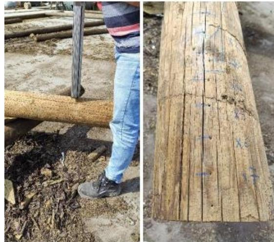
**Fig. 2.** Procedure to identify the degradation in the wooden poles **Fig. 3.** Measurements made with Resistograph
