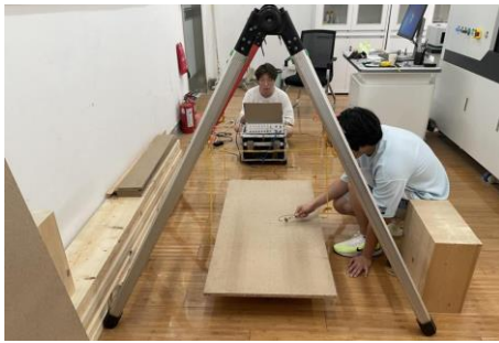
a. 1/4 board y-direction elastic modulus test
