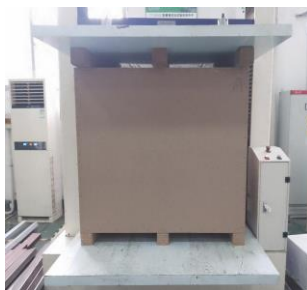
a. Stacking test methods using a static load
