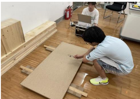
a. 1/4 board elastic modulus test
