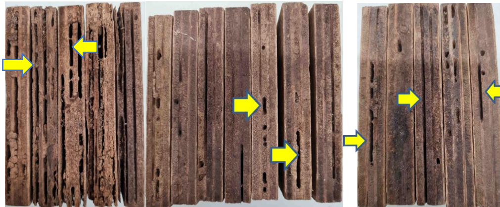
Fig. 3. Edgewise failure details on SWP and HWP specimens; While the surface veneers look intact, most damage was initiated from edges and progressed via core veneers where the retention of biocide was low.
