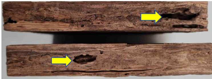
Fig. 6. Edgewise failure details on OSB specimens. In some cases, termite damage was initiated from edges of core sections of OSB specimens indicating full protection threshold level was not achieved even at those high retention areas.
