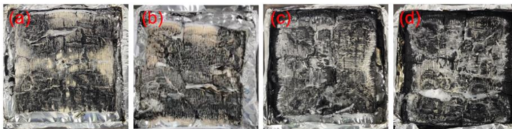
Fig. 12. The appearance of wood after burning: (a) U-PI, (b) D-PI, (c) FR-P, (d) D/FR-PI
