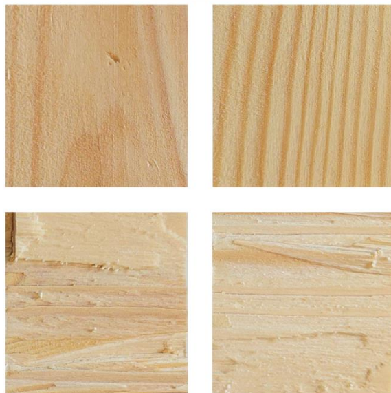
Fig. 9. Wood samples with 100% wood fracture (top) and 100% adhesive fracture (bottom)
