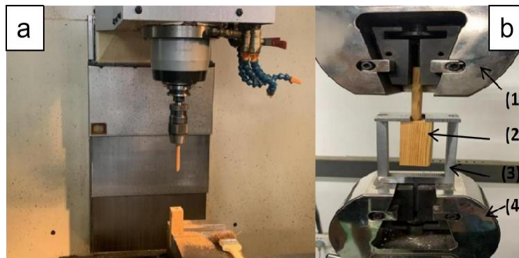
Fig. 1. Rotary friction welding test system. (a) Welding test rig; (b) Tensile test rig; (1) Tensile upper clamping block; (2) Wooden specimen; (3) Clamping fixture; (4) Tensile lower clamping block
