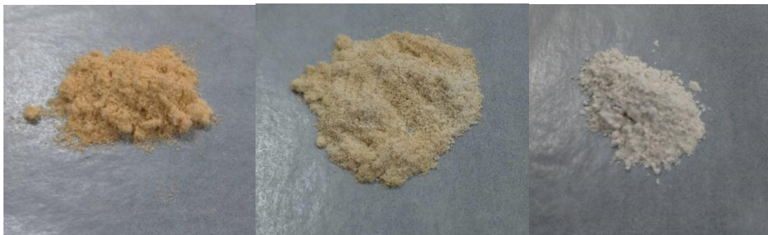
Fig. 1. Sample of wooden material (wood), wood mixed with montmorillonite, and montmorillonite
