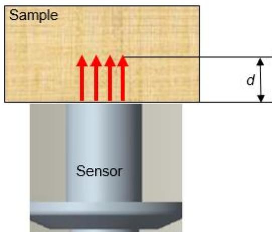
**Fig. 4.** Schematic representation of heat transfer from the sensor to the sample:  $d$  – depth of heat penetration into the sample
