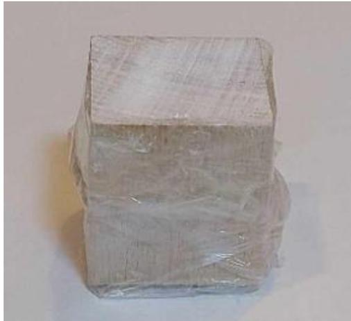
**Fig. 2.** Wood samples of dimensions of  $(3 \times 3 \times 3)$  cm<sup>3</sup> prepared for testing
