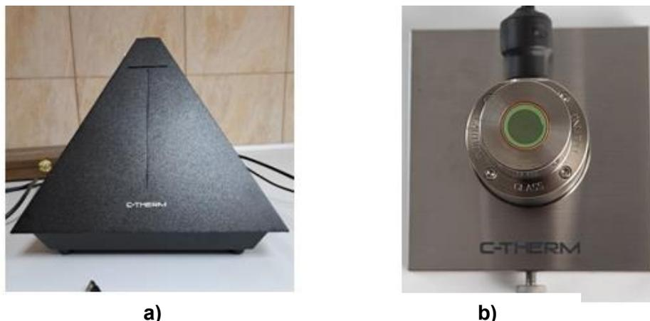
**Fig. 3.** Experimental setup for thermal effusivity and conductivity measurements: 3a: Thermal conductivity analyzer; 3b: Modified transient plane source sensor
