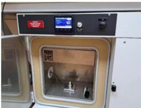
**Fig. 5.** Tenney environmental thermal chamber
