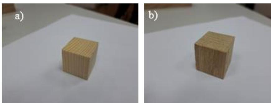
**Fig. 1.** Wood samples dimensions of  $(3 \times 3 \times 3)$  cm<sup>3</sup>: 1a: Beech wood samples; and 1b: Fir wood samples
