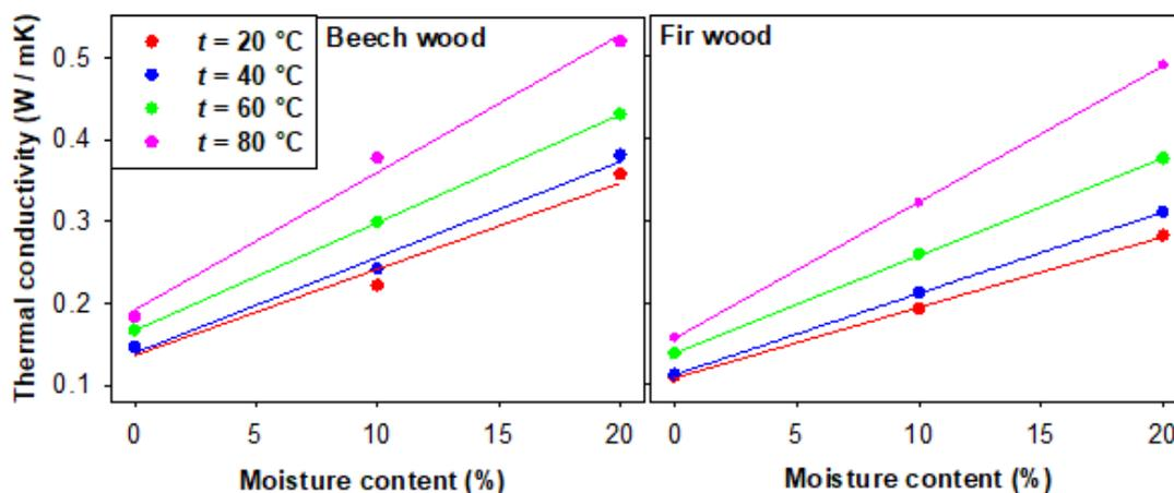
**Fig. 7.** Diagrams of the dependence of the mean value of thermal conductivity of beech and fir samples in the longitudinal direction on moisture content with associated regression curves at  $t = 20, 40, 60,$  and  $80\text{ }^{\circ}\text{C}$
