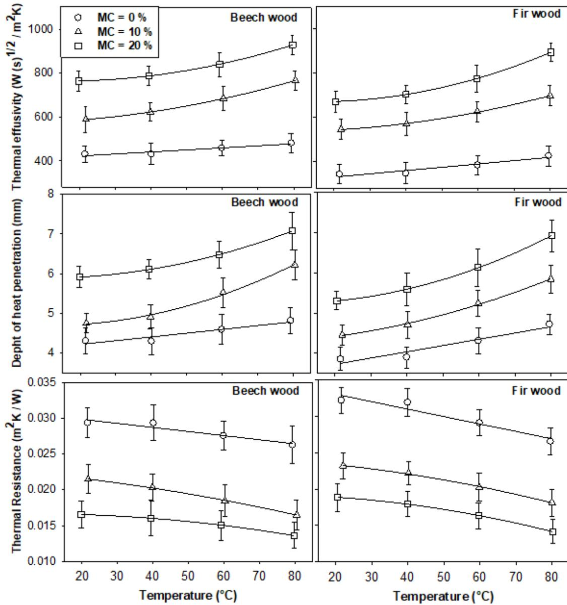
**Fig. A1.** Diagrams of the dependence of the mean value of thermal effusivity, depth of heat penetration and thermal resistance of beech and fir wood samples in the longitudinal direction on temperature with associated standard deviations and regression curves at moisture content of 0%, 10%, and 20%
