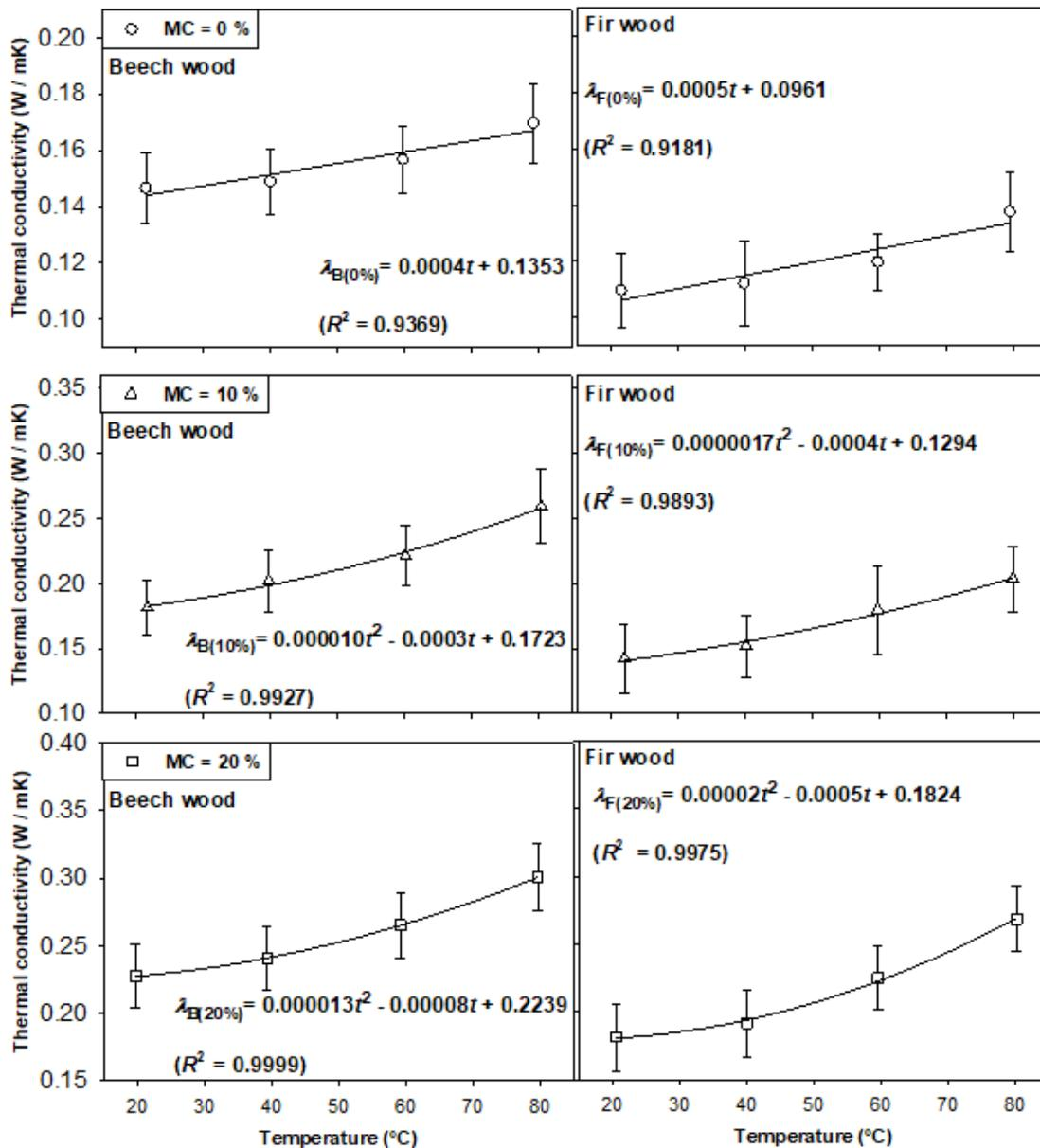
**Fig. 6.** Diagrams of the dependence of the mean value of thermal conductivity of beech and fir samples in the longitudinal direction on temperature with the associated standard deviations and regression curves at moisture content of 0%, 10%, and 20%
