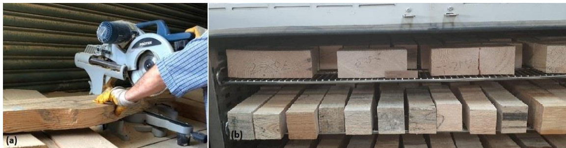
Fig. 4. (a) Moisture and density of sample cutting at the end of the test, and (b) oven drying for moisture content
