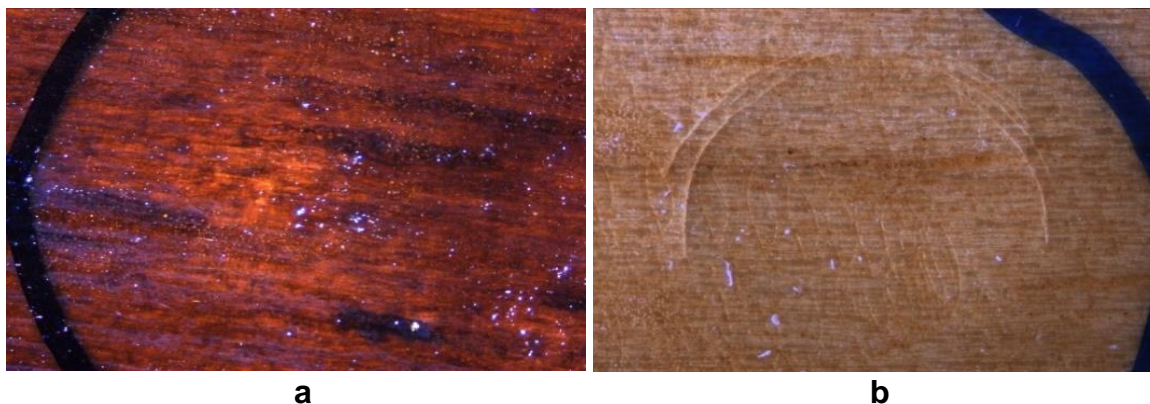
Fig. 5. Impact resistance of UPU (a) and BPU (b) coated wood
