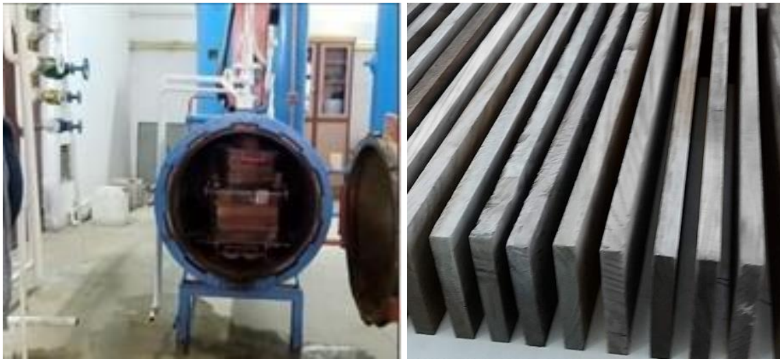
Fig. 2. Impregnation of test samples
