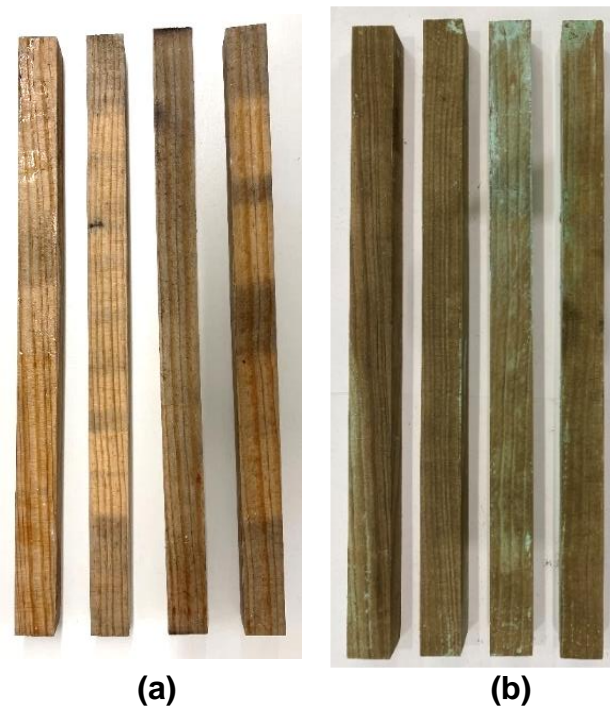
Fig. 5. Pine wood pieces after MW treatment (a) before and (b) after impregnation with the preservative product.
