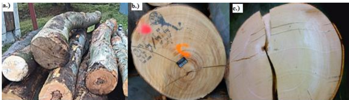
Fig. 4. Selections beech logs on yield a.) log with greatest curvature, b.) log with eccentric pith, c.) shiny appearance after drying in disks.
