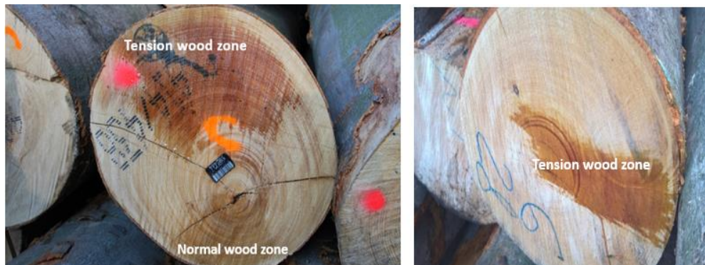
Fig. 6. Application of reagent on the log yard on surface of logs (Temperature was below zero)
