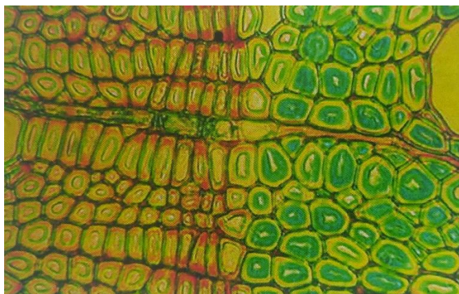
Fig. 2. Colour differentiation of the presence of normal wood red color and reaction wood green color based on the use of safranin and light green Kúdela and Čunderlík 2012).
