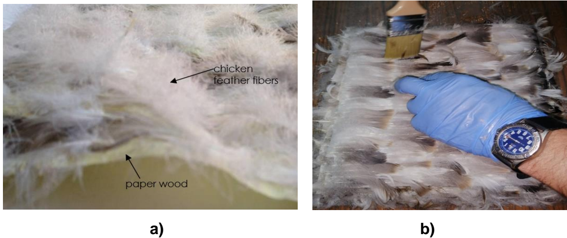
Fig. 1. a) A detail regarding the composition of a lamina, highlighting the wood paper and chicken feathers; b) The method of applying resin to consolidate the ten laminae
