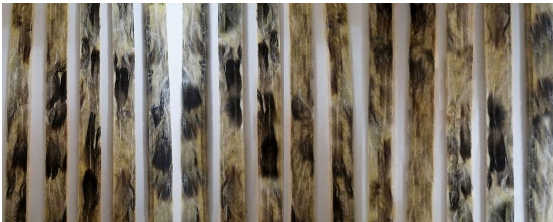
Fig. 3. An example with the 15 specimens cut for the tensile test from the T WCDE60 group
