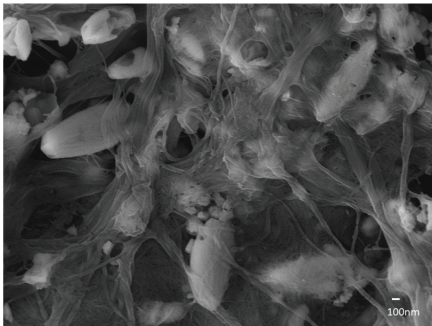
Figure 10. Scanning electron micrograph of co-processed MFC and precipitated calcium carbonate (PCC).
