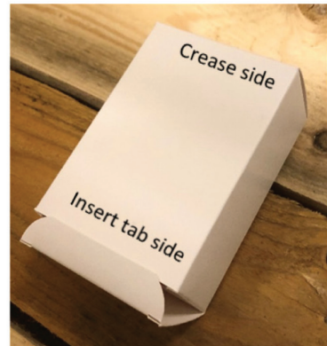
Figure 1. Left: Sketch of the package blank with drawing directions illustrated. A = 78 mm, B = 50mm, H = 110 mm. A MD crease is in this paper defined as a crease line perpendicular to the MD direction, e.g. a crease line along the long side of the package. A CD crease is correspondingly defined as a crease line perpendicular to the CD direction. Right: Erected package with insert tab not tucked in for illustration of non-symmetry.
