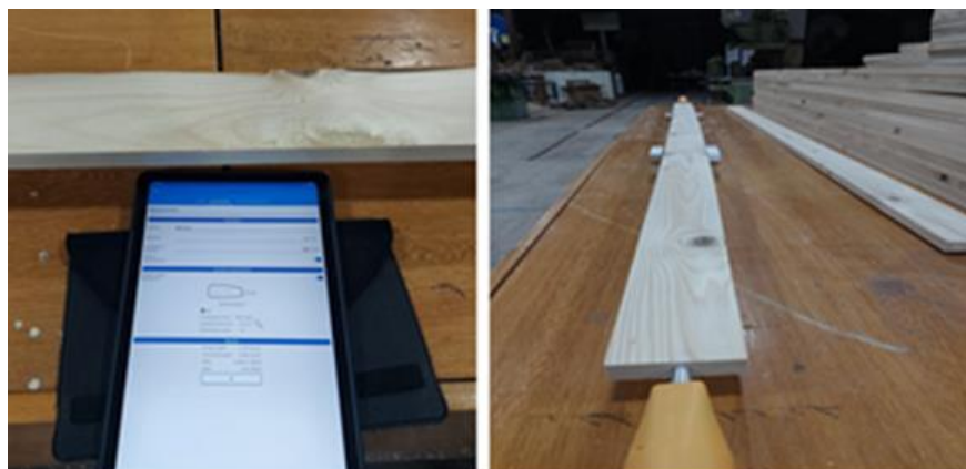
Fig. 1. Determining the strength classes of timber with an acoustic testing device
