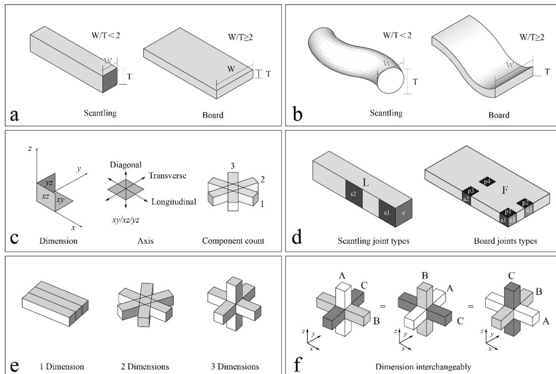
**Fig. 2.** MT joint coding. (a) Categories of scantlings and boards based on their cross-sectional dimensional ratios; (b) Curved components classification; (c) Definition of dimension, axis and component count; (d) Joint types; (e) Component joint by different dimensions; (f) Dimension interchangeably
