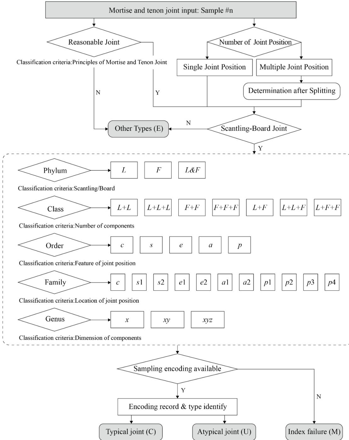
**Fig. 5.** Validation method for MT sampling, coding, and classification
