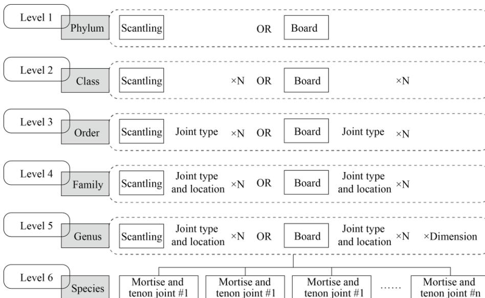
**Fig. 1.** The hierarchical structure of MT joints
