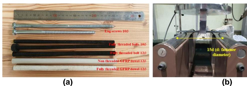
**Fig. 1.** Mechanical fasteners and setup of three-point bending test**Table 2.** Characteristics of Bending Strength of the Fasteners
