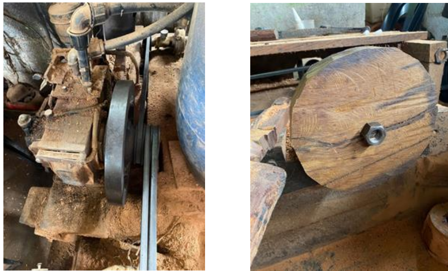
Fig. 3. The lathe machine for turning the wood into circular shape
