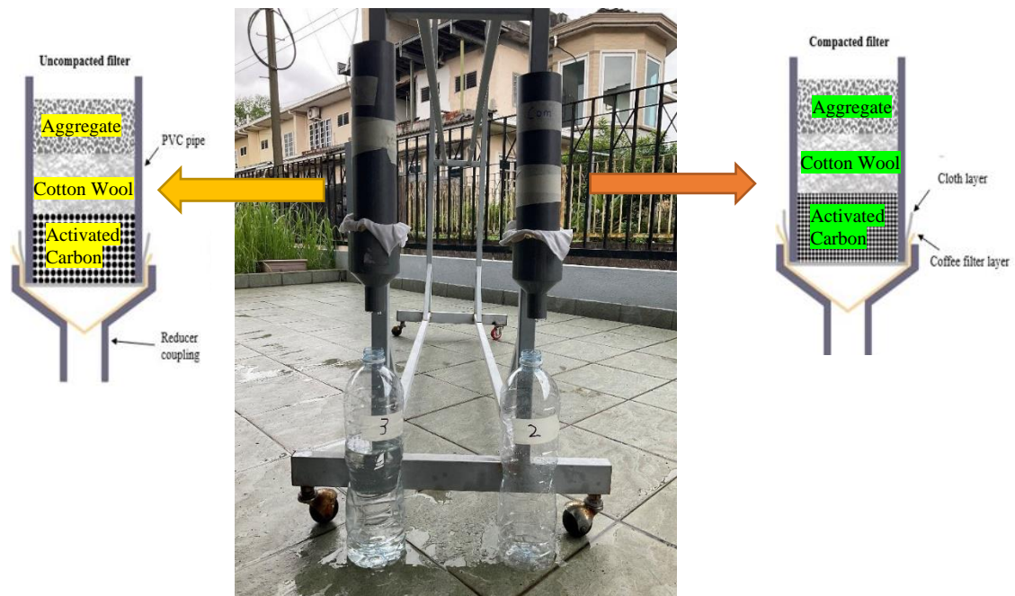
b) Filter assemblies for the two types
