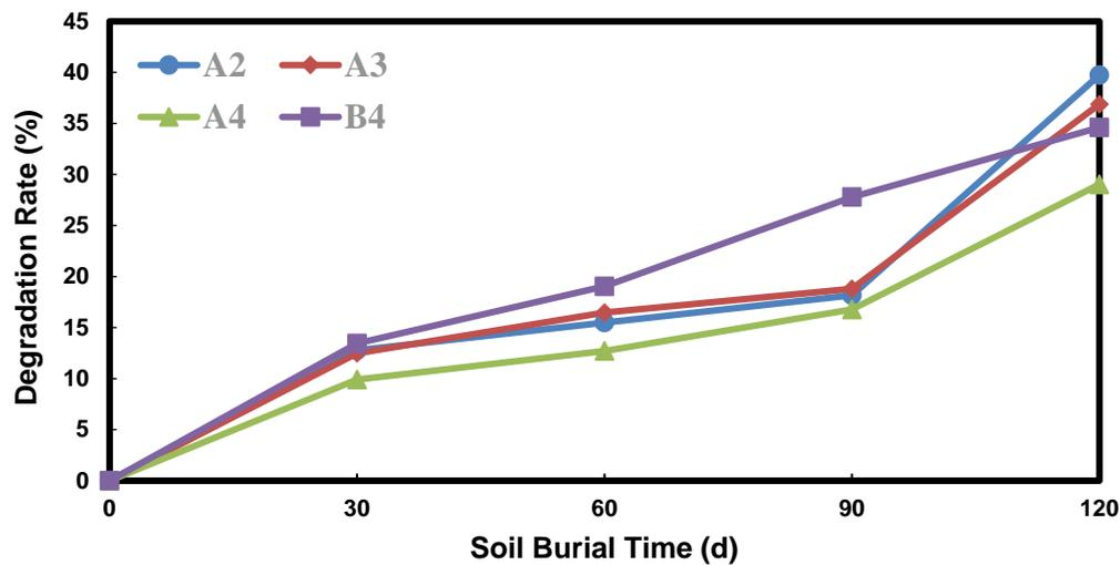
Fig. 11. Biodegradation curves of sugarcane leaf-based mulch samples
