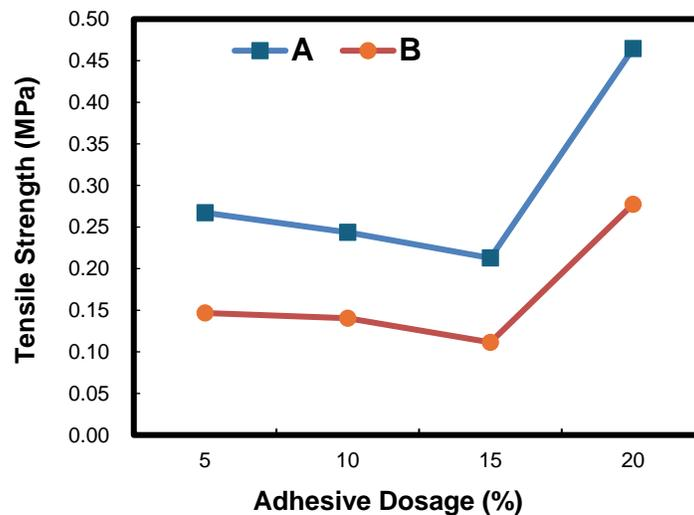
**Fig. 2.** Tensile strength of sugarcane leaf-based mulch samples prepared with different adhesives at different addition amounts
