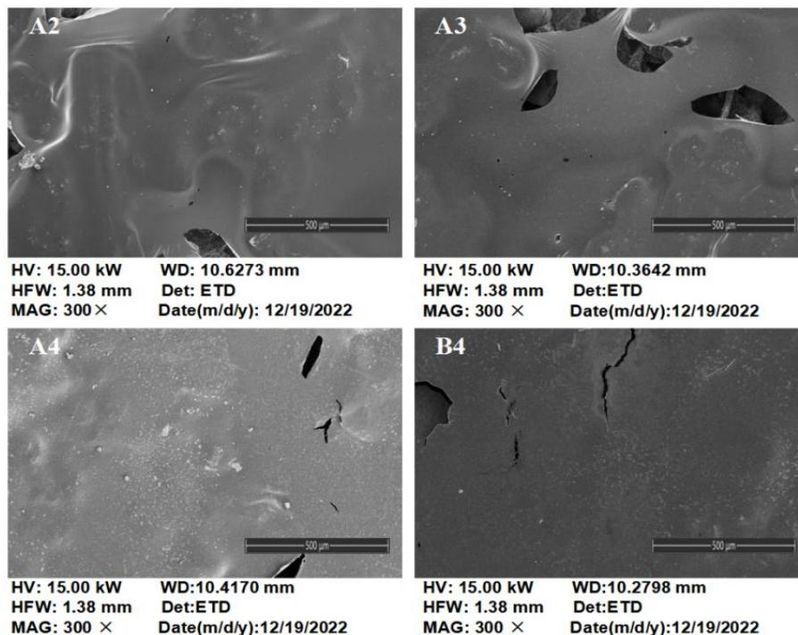
**Fig. 6.** Microstructure of the mulch surface before degradation
