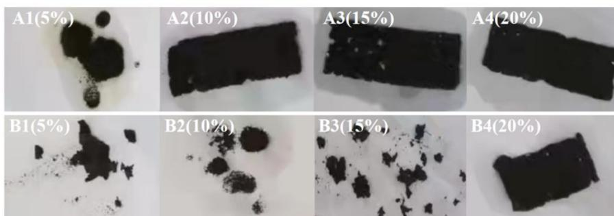
**Fig. 5.** Apparent morphology of swelling test for sugarcane leaf covering materials
