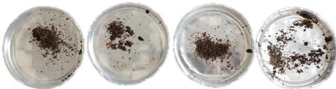
Fig. 12. Sugarcane leaf-based mulch samples buried in soil for 120 days (A2, A3, A4 and B4 from left to right)
