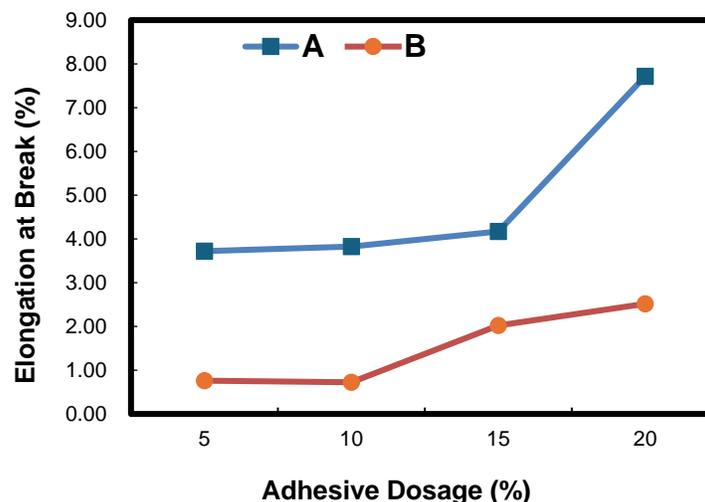
**Fig. 3.** Elongation at break of sugarcane leaf-based mulch samples prepared with different adhesives at different addition amounts
