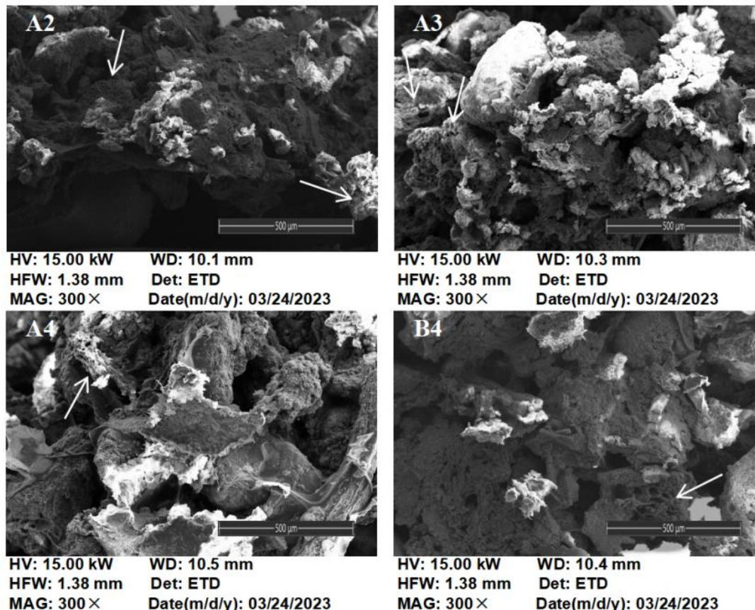
**Fig. 9.** Cross-sectional microstructure of the mulch after degradation
