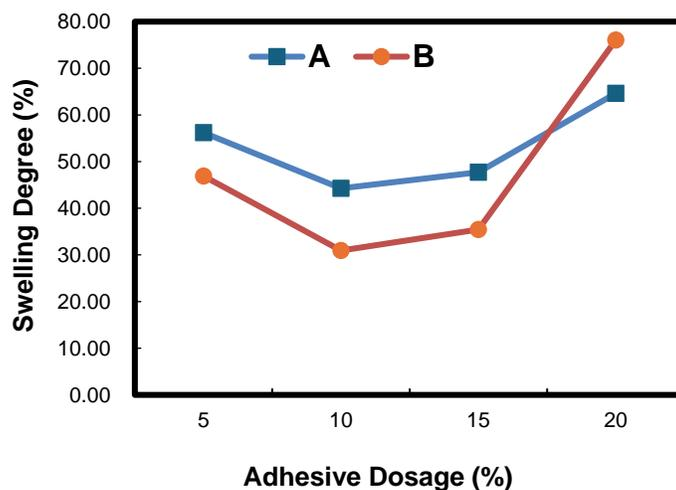
**Fig. 4.** Swelling degrees of sugarcane leaf-based mulch samples prepared with different adhesives at different addition amounts
