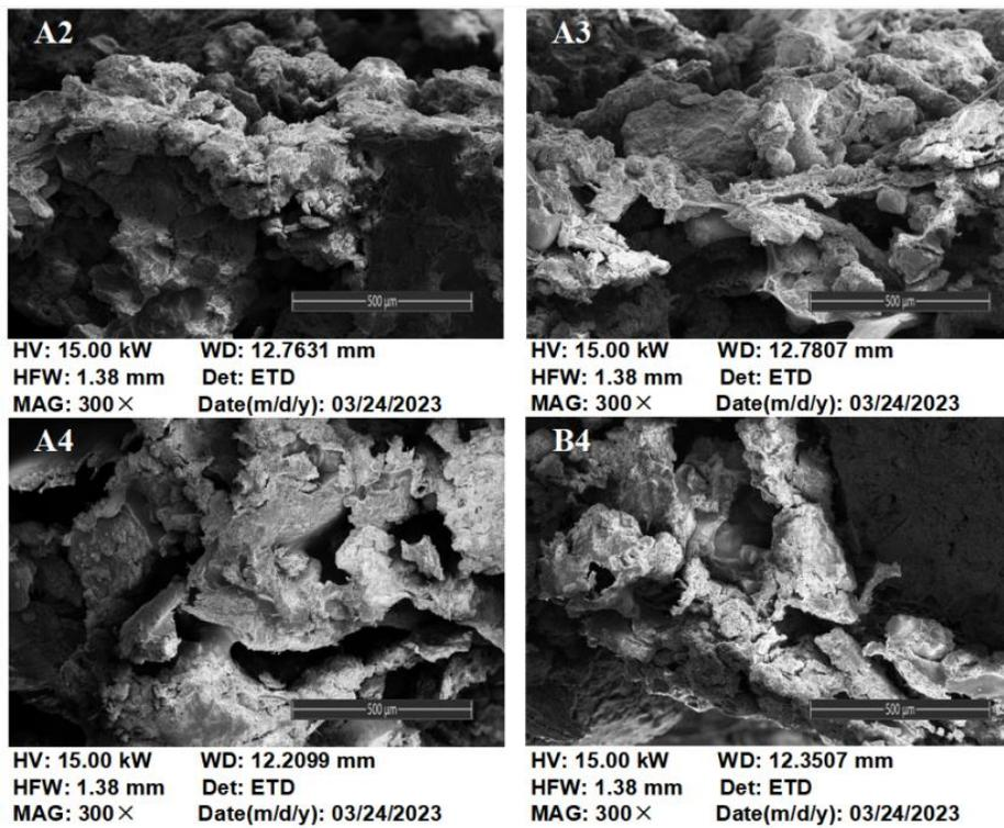
**Fig. 8.** Cross-sectional microstructure of the mulch before degradation
