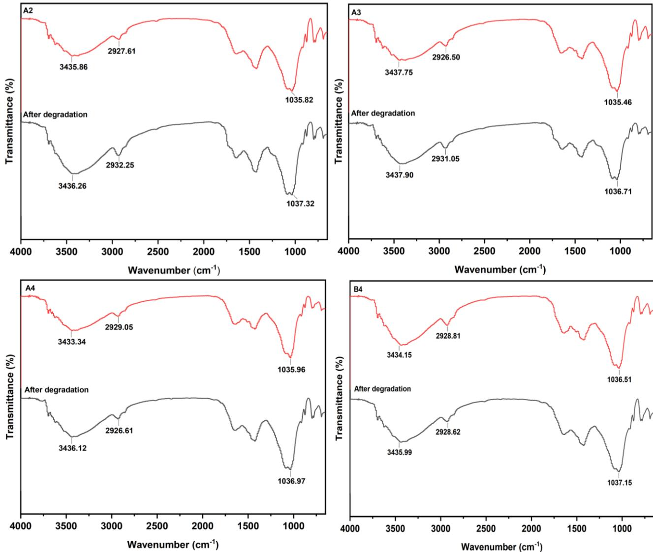
**Fig. 10.** Infrared absorbance spectra of covering materials before and after degradation
