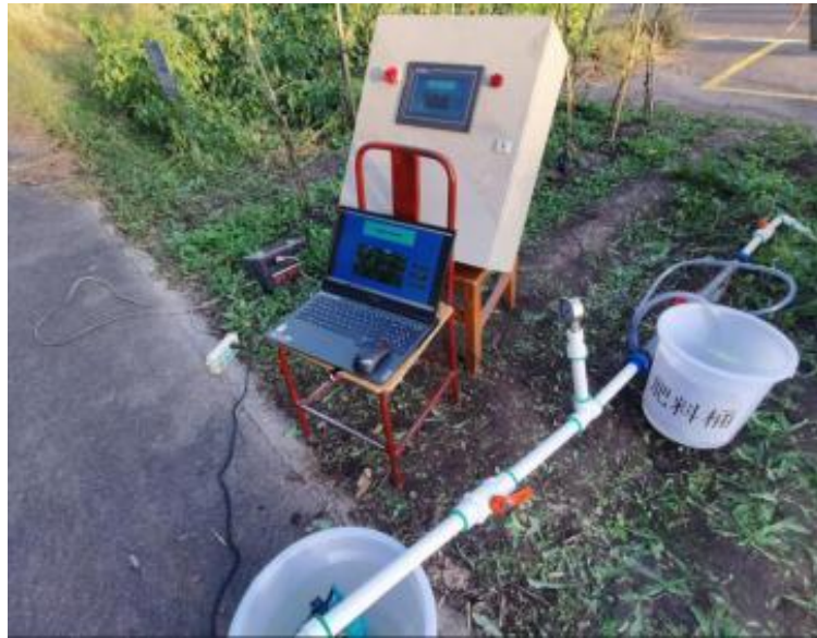
Fig. 11. Commissioning of the maize growth control system
