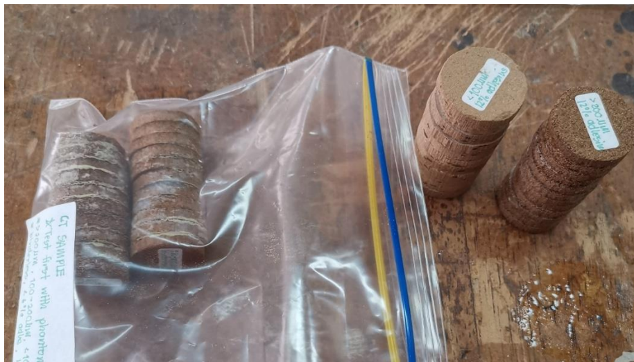
Fig. 4. Fabricated plug phantom at different percentages of adhesives and different particle sizes
