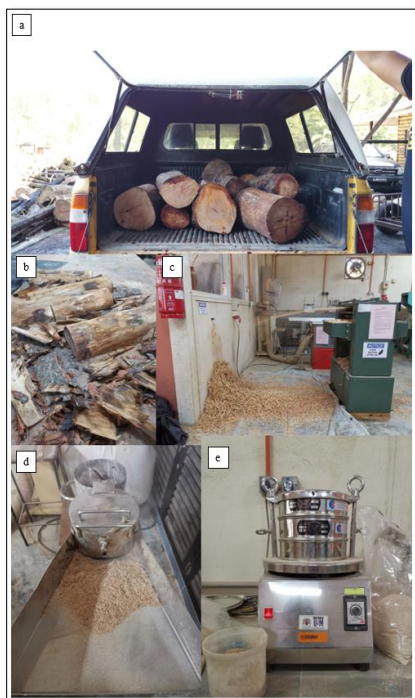
Fig. 2. (a) Wood truck collected from mangrove factory; (b) Debarking process of the wood trunk; (c) Planing process to produce wood particles; (d) Wood particle underwent grinding process; (e) Sieving process to prepare the wood particles at different particle sizes
