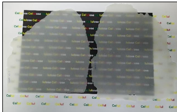
Fig. 6. Visual representation of finalized dry nanopapers derived from BHKP-EH-5K samples, showcasing the sequential process of their formation at 15% consistency, mechanical pressing to over 90% solids, subsequent oven drying, and equilibration to achieve a stable 95% solids content.
