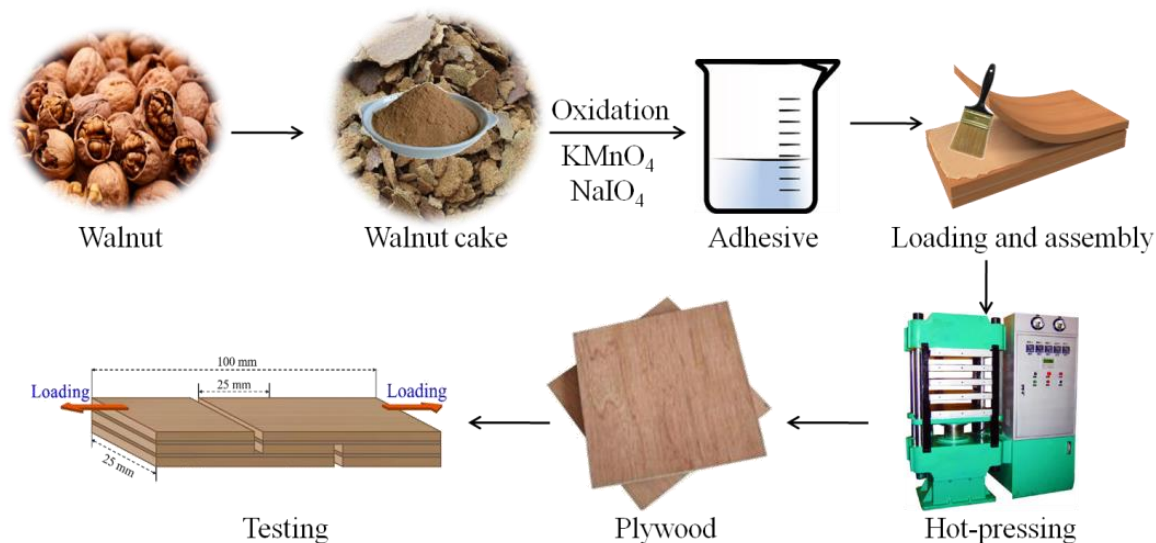
Fig. 1. Diagram of adhesive preparation and plywood preparation and testing
