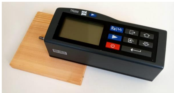
Fig. 3. Surface roughness measurement device
