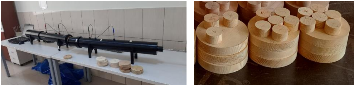
Fig. 4. Impedance tubes and test samples
