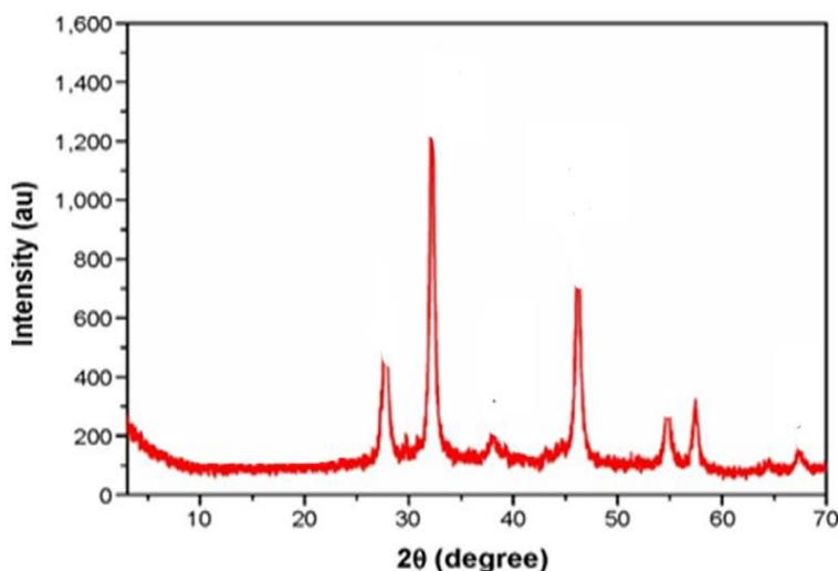
Fig. 8. X-ray diffraction analysis of prepared silver-PLA nanocomposite material
