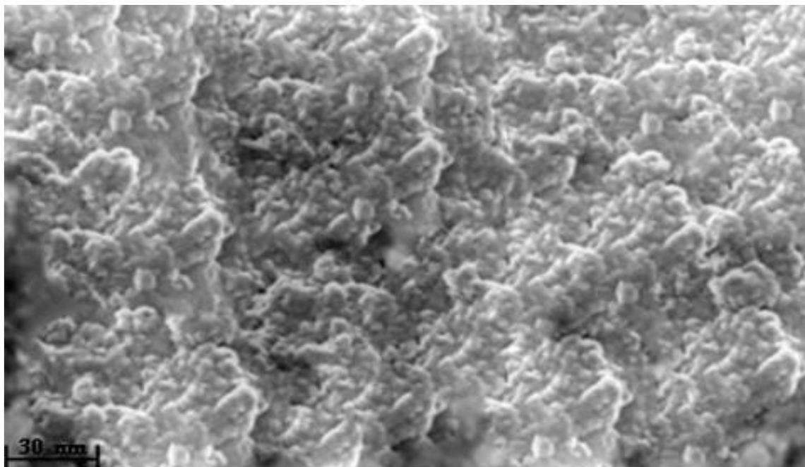
Fig. 9. SEM Images of Ag/PLA nano composite material
