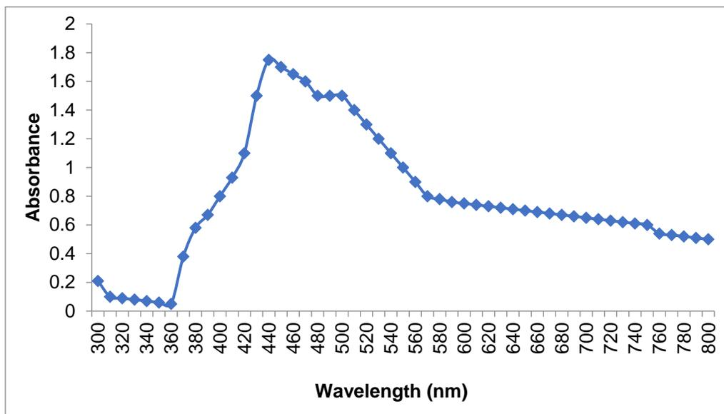
Fig. 7. UV-visible absorbance spectra of Ag/PLA nano composite material
