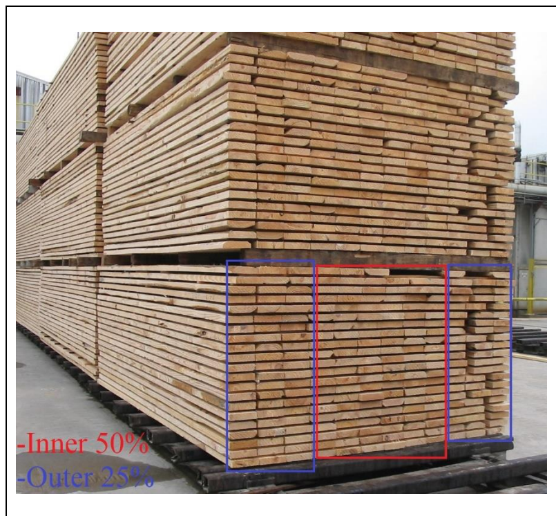
Fig. 1. Exemplar packages of 2 in. (5-cm) thick pine lumber, stacked on sticker, awaiting drying at a commercial kiln
