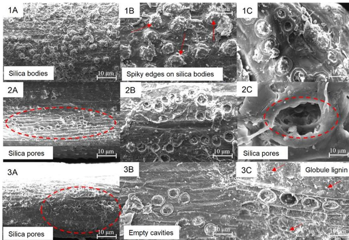
**Fig. 9.** Surface morphologies *via* SEM of PES (1A, 1B, and 1C), AAP-PES (2A, 2B, and 2C), and AAPB-PES (3A, 3B, and 3C) at 250X, 700X, 1000X, and 5000X magnifications
