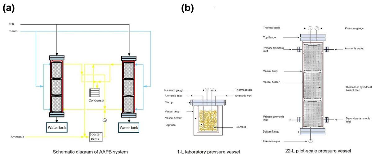
**Fig. 2.** (a) The schematics of pilot scale diagram of batch AAP (AAPB) system, (b) Configuration of laboratory and pilot scale pretreatment vessels
