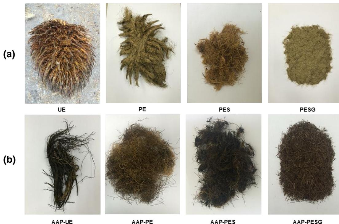
**Fig. 4.** Physical structures of: (a) untreated EFB, and (b) pretreated EFB
