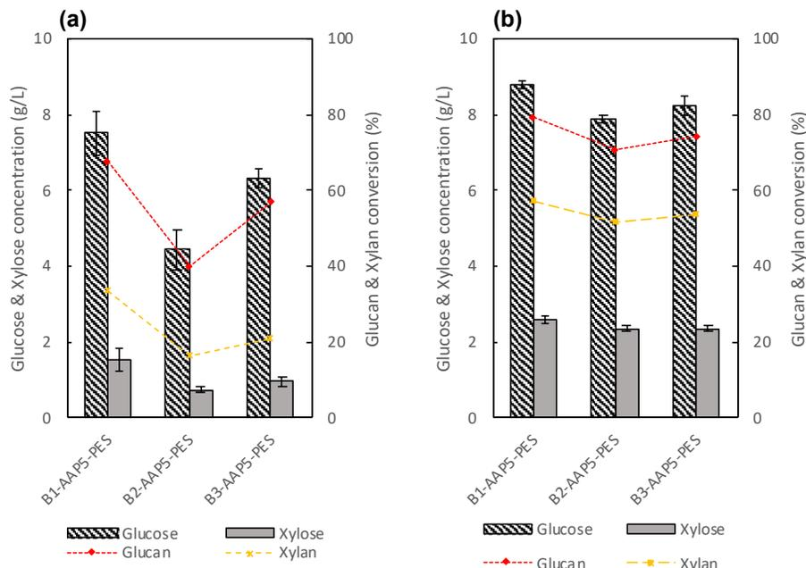
**Fig. 10.** Enzymatic hydrolysis of (a) AAPB-T3 and (b) AAPB-T4 at 1% glucan loading for each cylindrical basket filters
