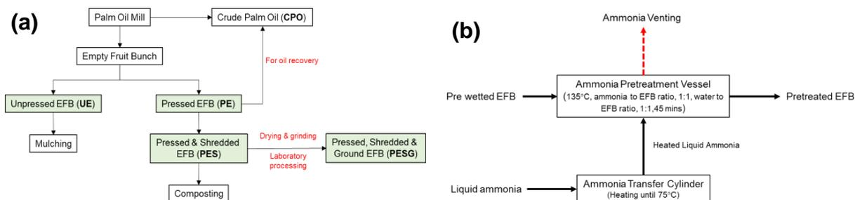
**Fig. 1.** (a) Flow of different categories of EFB samples from oil palm mill, (b) Schematic diagram of anhydrous ammonia pretreatment process
