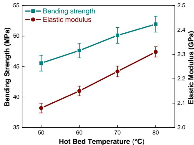
Fig. 5. Effect of hot bed temperature on the bending properties of ABS specimens
