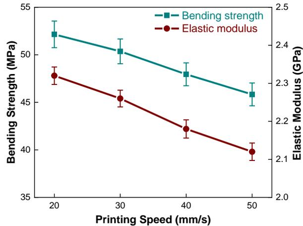
Fig. 3. Effect of printing speed on the bending properties of ABS specimens
