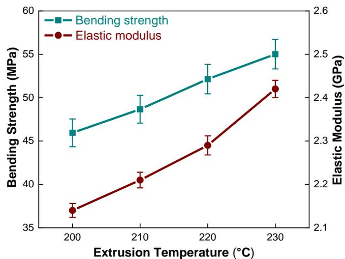
Fig. 4. Effect of extrusion temperature on the bending properties of ABS specimens
