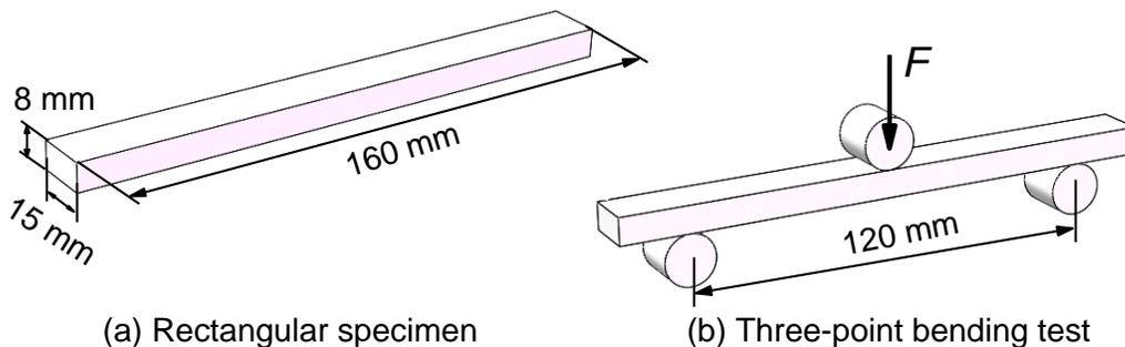
Fig. 2. Rectangular specimen and three-point bending test
