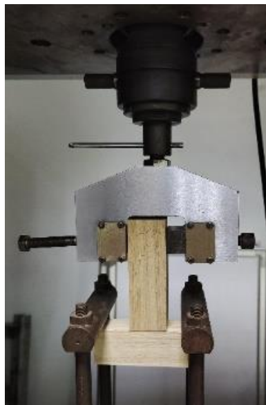
Fig. 4. Schematic diagram of specimen clamping
