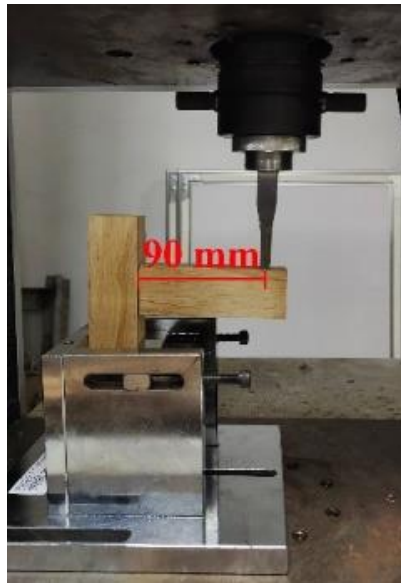
Fig. 5. Schematic diagram of specimen clamping
