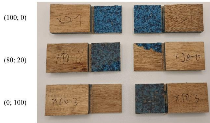
Fig. 3. The calculation method of core layer failure rate and adhesive layer failure rate
