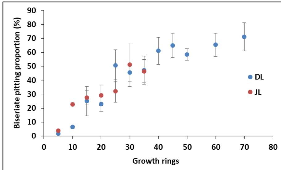
**Fig. 8.** Radial variation of the proportion of the tracheids with biseriate bordered pitting in earlywood of DL and JL
