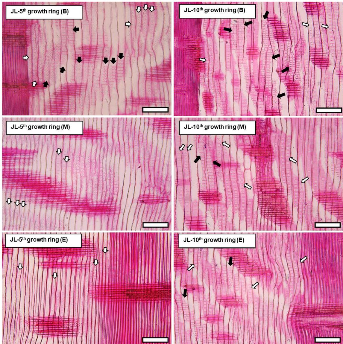
**Fig. 5.** Optical micrographs of the radial sections in the beginning (B), middle (M), and end (E) parts of earlywood of the 5<sup>th</sup> and 10<sup>th</sup> growth ring in JL. White arrows indicate uniseriate bordered pitting, while black arrows indicate biseriate pitting. Scale bars: 200  $\mu$ m
