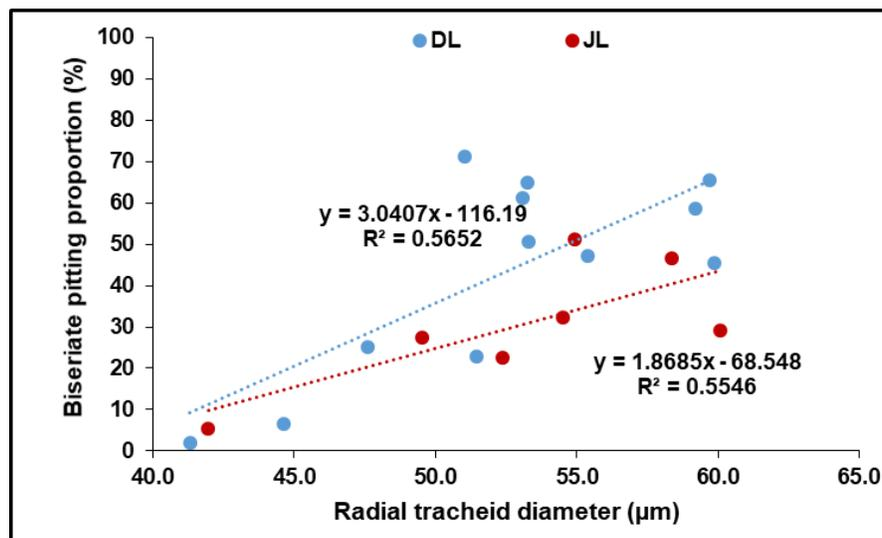
**Fig. 10.** Relationships between the earlywood tracheid width and the tracheid proportion with biseriate pitting in Dahurian larch (DL) and Japanese larch (JL) woods. The dotted line indicates the mean value of both species.
