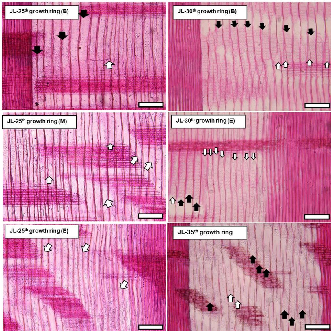
**Fig. 7.** Optical micrographs of the radial sections in the beginning (B), middle (M), and end (E) parts of earlywood of the 25<sup>th</sup>, 30<sup>th</sup>, and 35<sup>th</sup> growth ring in JL. White arrows indicate uniseriate bordered pitting, while black arrows indicate biseriate pitting. Scale bars: 200  $\mu$ m
