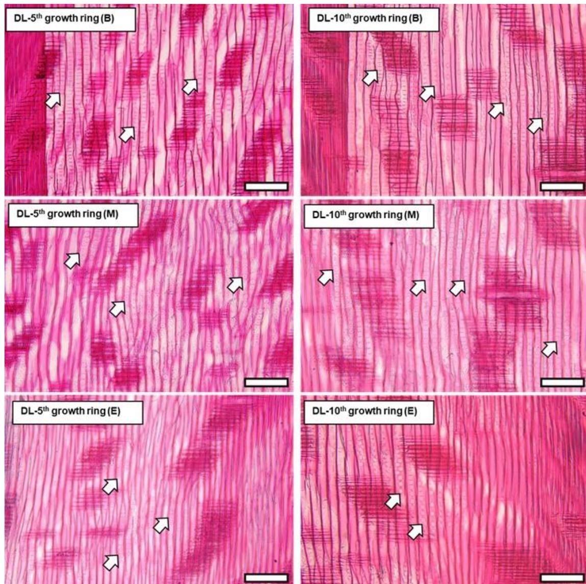
**Fig. 2.** Optical micrographs of the radial sections in the beginning (B), middle (M), and end (E) parts of earlywood at the 5<sup>th</sup> and 10<sup>th</sup> growth ring in DL. The white arrows indicate the tracheids with predominantly uniseriate bordered pitting. Scale bars: 200  $\mu$ m
