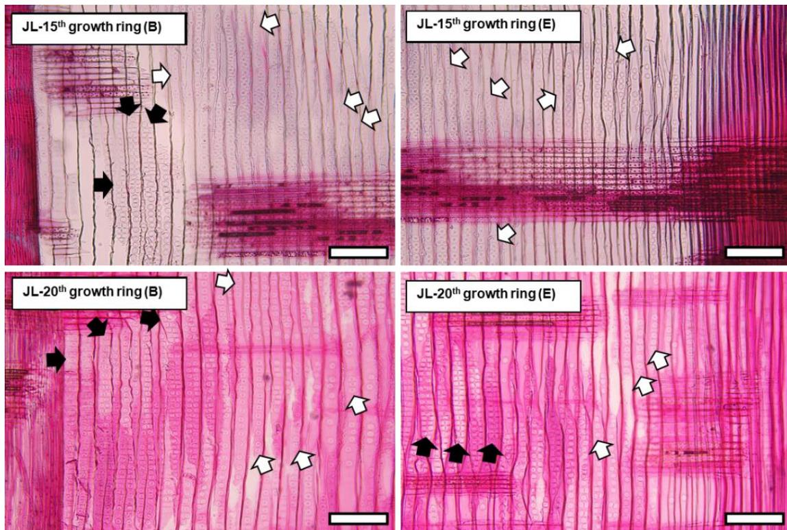
**Fig. 6.** Optical micrographs of the radial sections in the beginning (B) and end (E) parts of earlywood of the 15<sup>th</sup> and 20<sup>th</sup> growth ring in JL. White arrows indicate uniseriate bordered pitting, while black arrows indicate biseriate pitting. Scale bars: 200  $\mu$ m
