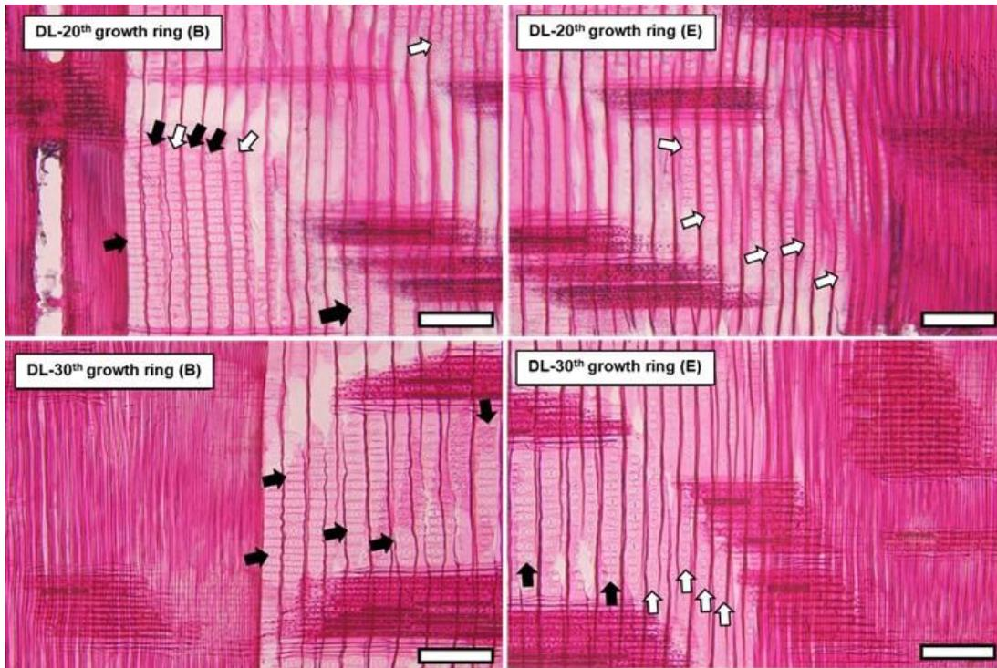
**Fig. 3.** Optical micrographs of the radial sections in the beginning (B) and end (E) parts of earlywood at the 20<sup>th</sup> and 30<sup>th</sup> growth ring in DL. White arrows indicate the tracheids with predominantly uniseriate bordered pitting, while black arrows indicate the tracheids with predominantly biseriate pitting. Scale bars: 200  $\mu$ m
