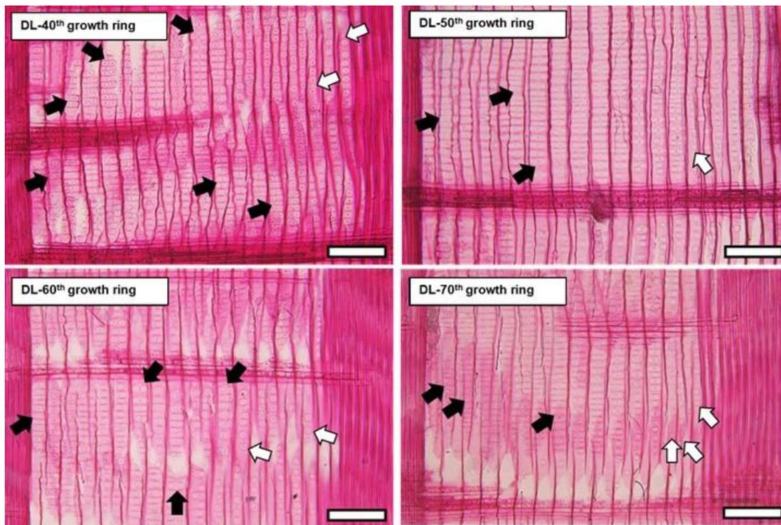
**Fig. 4.** Optical micrographs of the radial sections in the 40<sup>th</sup>, 50<sup>th</sup>, 60<sup>th</sup>, and 70<sup>th</sup> growth ring in DL. White arrows indicate uniseriate bordered pitting, while black arrows indicate biseriate pitting. Scale bars: 200  $\mu$ m
