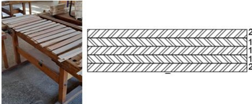
Fig. 1. Arrangements of lamellas in laminated timber: 1-willow wood; 2- willow, ash or yellow pine wood.
