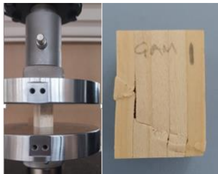
Fig. 2. Pressure testing of laminated timbers
