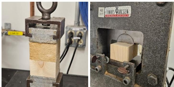
**Fig. 3.** Tensile perpendicular-to-grain testing (left) and shear testing (right) with a WFI:SPF Sample
