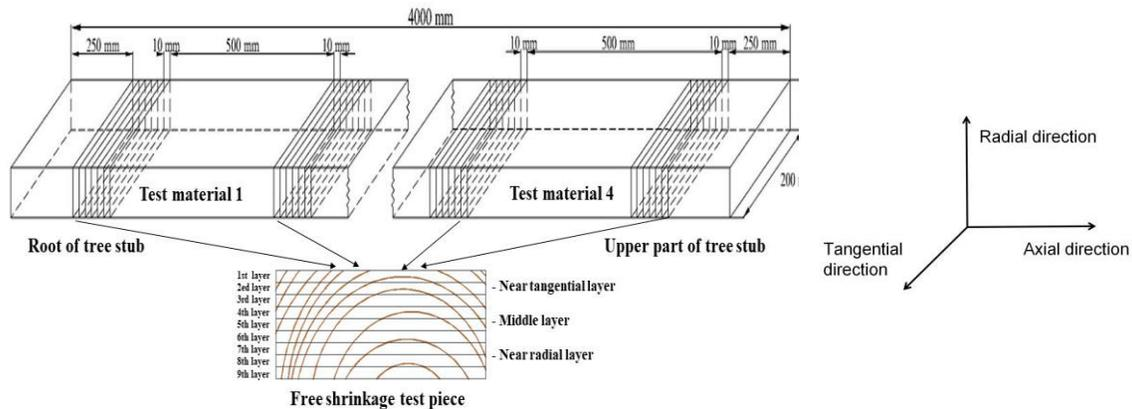
**Fig. 1.** Preparation of experimental specimens for studying the free and actual shrinkage patterns of *Pinus sylvestris* var. *mongolica* lumber (Zhu *et al.* 2021; [CC BY 4.0](https://creativecommons.org/licenses/by/4.0/) license)
