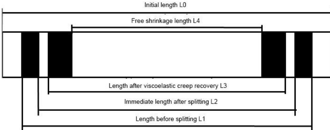
**Fig. 2.** Measurement of various strains during the drying process of *Pinus sylvestris* var. *mongolica* specimens
