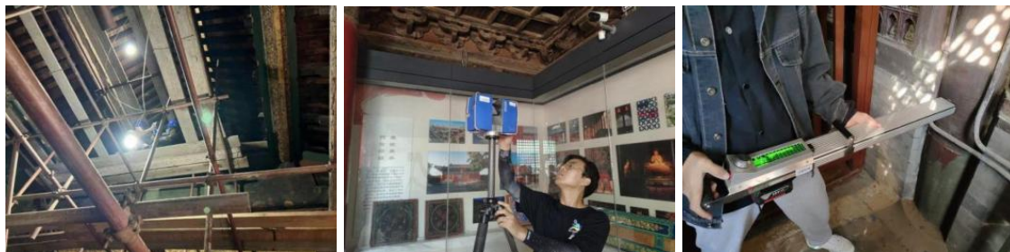
Fig. 5. Zhihua Temple 3D laser scanning and impedance analyzer testing
