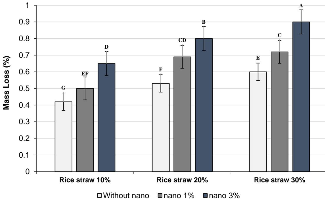
**Fig. 11.** Effect of rice straw mix ratio, gypsum, and BNCf on mass loss of composites
