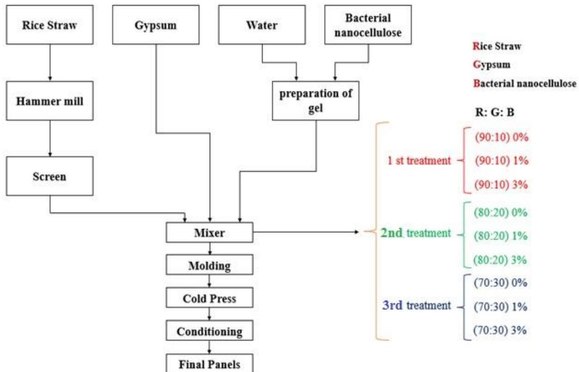
**Fig. 4.** The process of making rice straw and gypsum composite board
