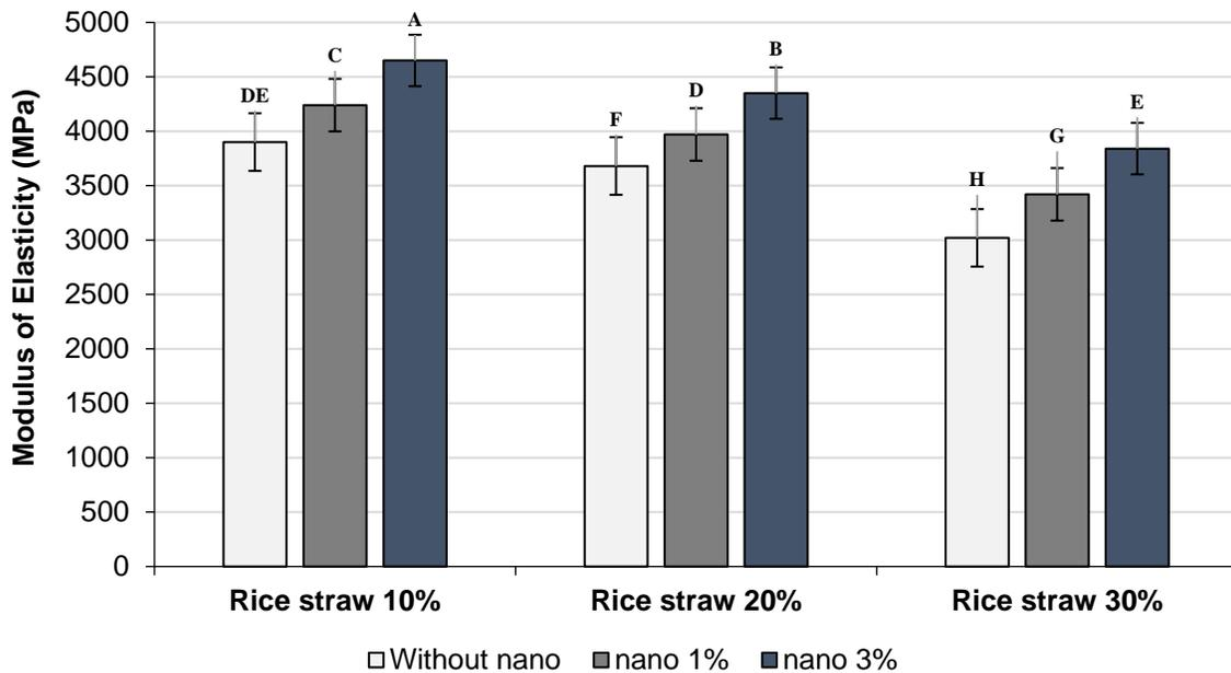
**Fig. 7.** Effect of rice straw mix ratio, gypsum, and BNCF on modulus of elasticity of composites
