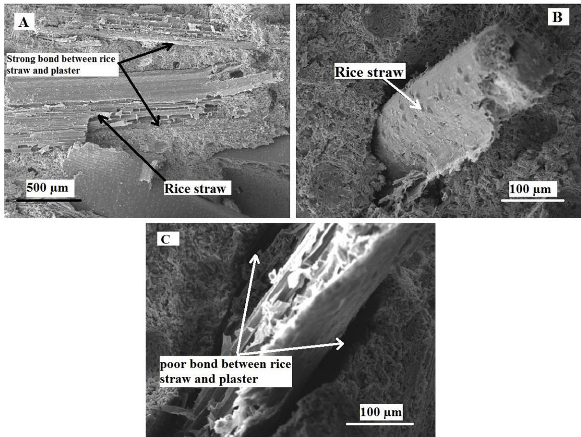
**Fig. 12.** SEM images of refractive surfaces, A: Boards containing 3% bacterial nanocellulose fiber, B: Boards containing 1% bacterial nanocellulose, and C; Boards without- bacterial nanocellulose (c)
