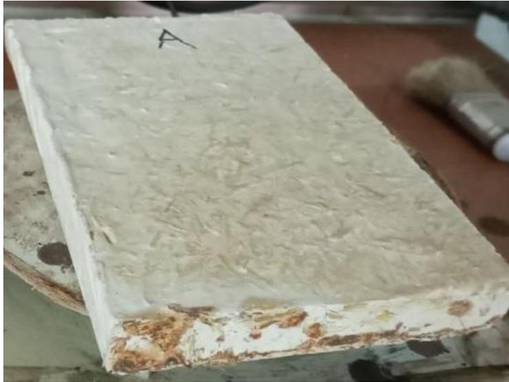
**Fig. 3.** Board made of rice straw and gypsum
