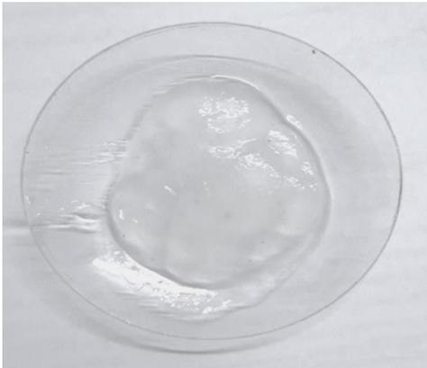
**Fig. 2.** Bacterial nanocellulose fiber used in this research*Sample preparation*
