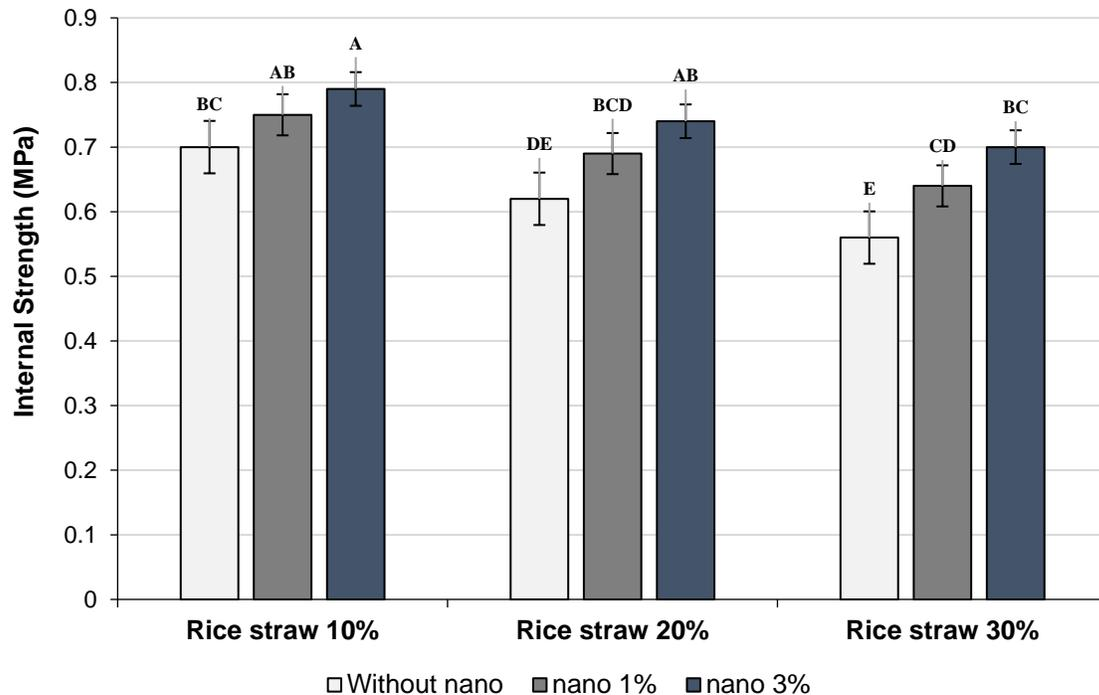
**Fig. 8.** Effect of rice straw mix ratio, gypsum, and BNCF on internal strength of composites
