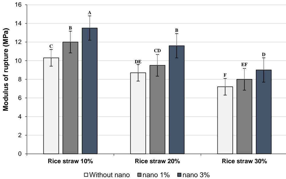
**Fig. 6.** Effect of rice straw mix ratio, gypsum, and bacterial nanocellulose fiber (BNCF) on modulus of rupture of composites
