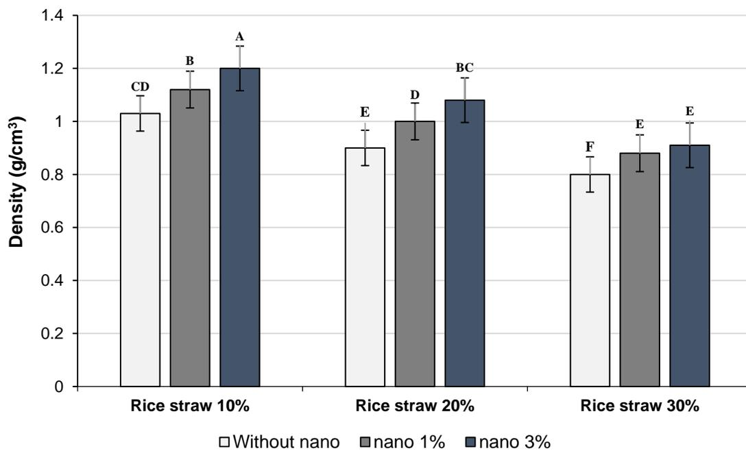
**Fig. 10.** Effect of rice straw mix ratio, gypsum, and BNCf on density of composites
