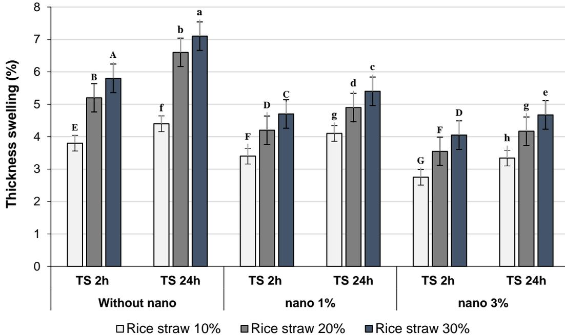
**Fig. 9.** Effect of rice straw mix ratio, gypsum, and BNCf on thickness swelling after 2 h and 24 h immersion in water of composites
