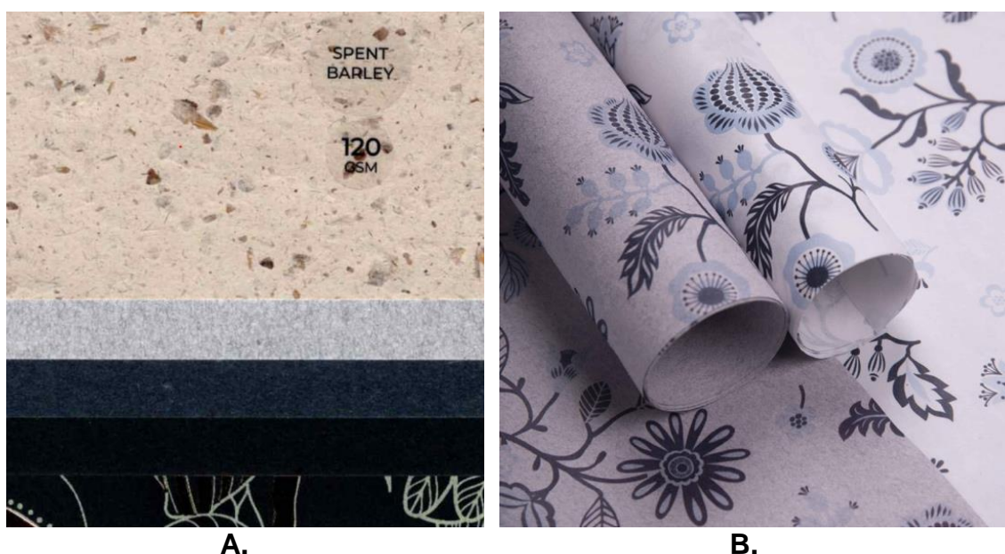
Fig. 2. A range of Bluecat paper products. A: sample-book items, including some with agricultural residues and denim; B: Gift wrapping paper (after printing) made from grey textile offcuts
