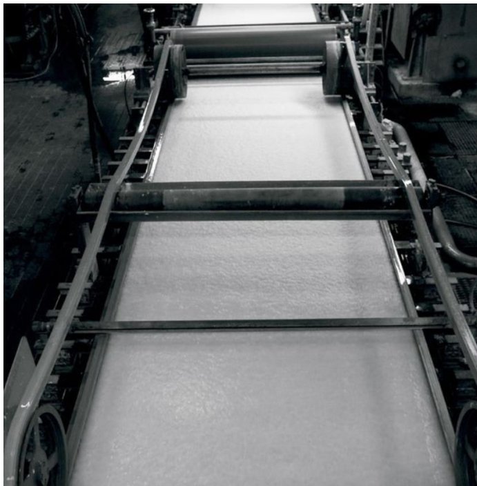
Fig. 1. Fourdrinier section of the new paper machine system
