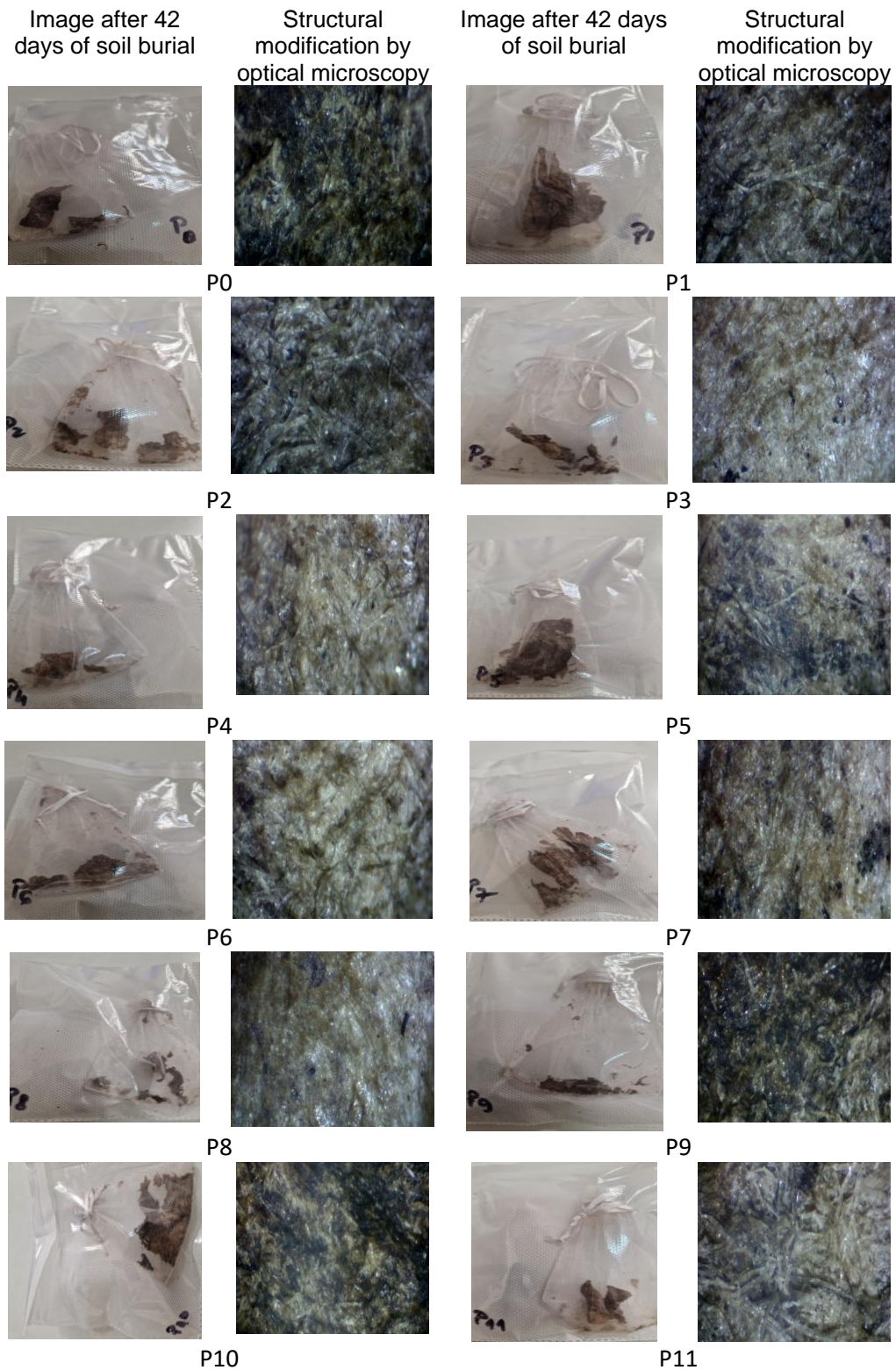
Fig. 12. Physical appearance of the polysaccharides coated papers after being buried in soil
