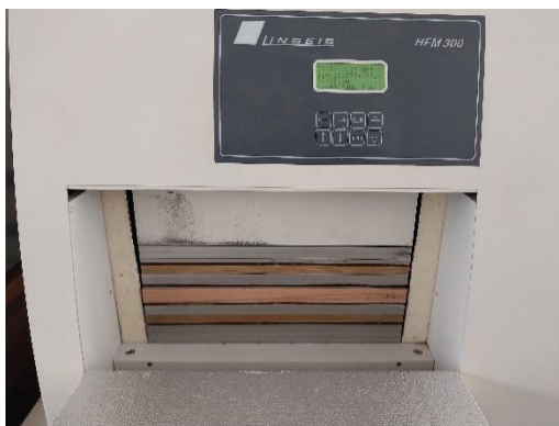
Fig. 3. Thermal conductivity device used in test measurements
