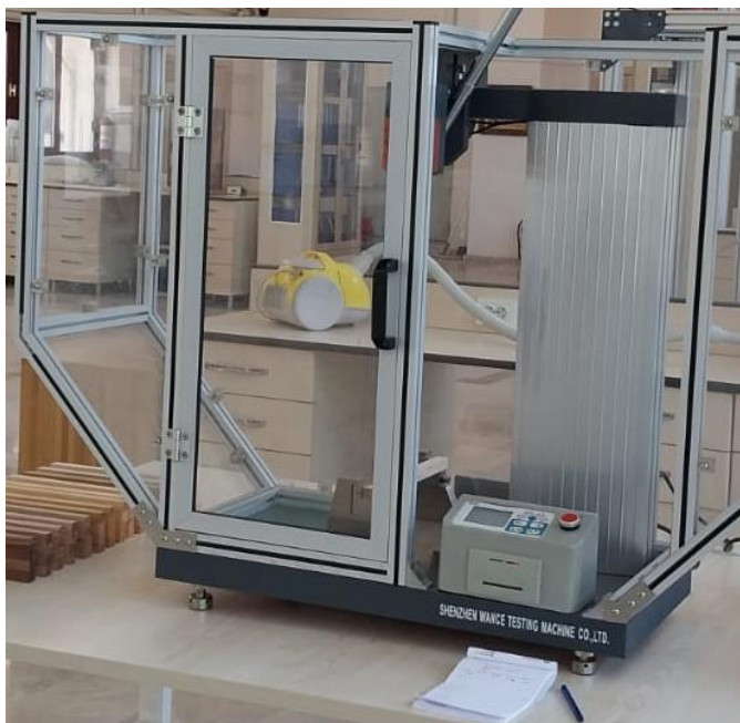
Fig. 1. IBS test device used in test measurements
