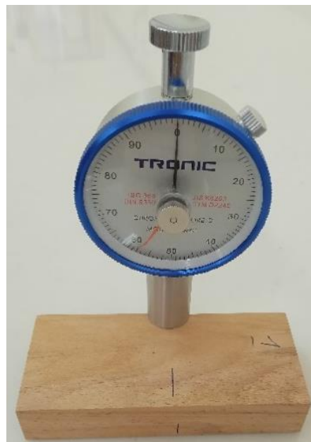
Fig. 2. Shore-D hardness device used in test measurements
