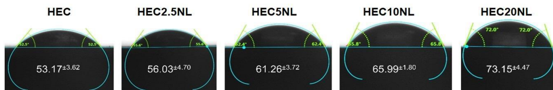
Fig. 4. Water contact angle for the composite films. All the values are expressed as an average of 10 measurements \pm one standard deviation.
