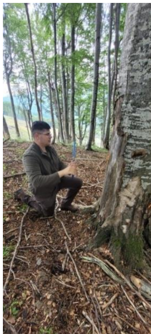
Fig. 7. The growth core extraction using the Pressler drill
