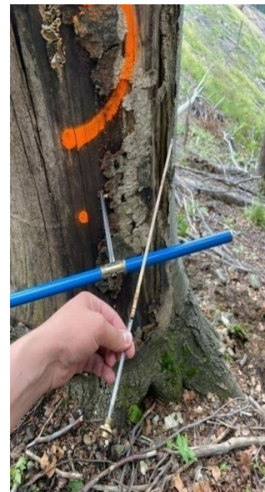
Fig. 8. The extracted growth core
