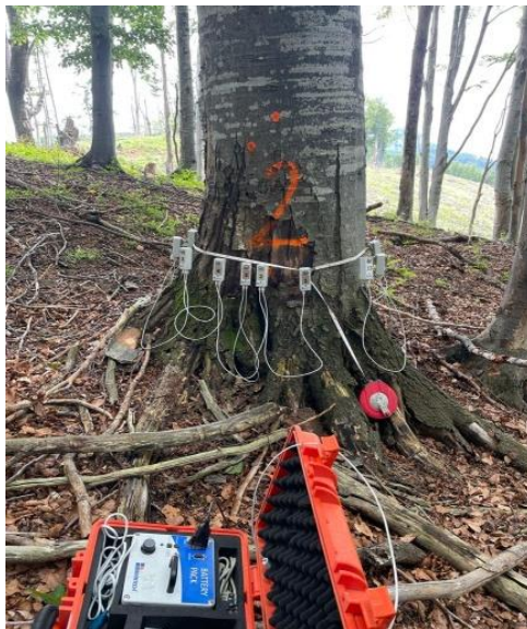
Fig. 5. The ArbotomRinntech tomograph and the sensors connection
