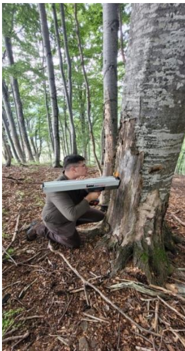
Fig. 6. The investigations made by the IML F-500 RESI resistograph
