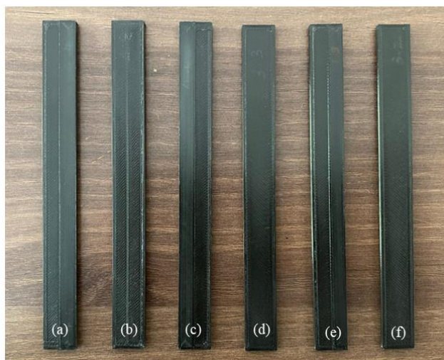
Fig. 6. Flexural test specimen (a) 0% reinforcement, (b) 10% reinforcement, (c) 20% reinforcement, (d) 30% reinforcement, (e) 40% reinforcement, and (f) 50% reinforcement
